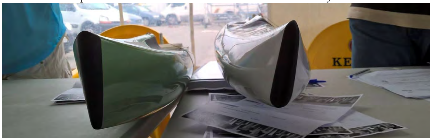
Bow comparison: The thinking obviously changed significantly from Kantun S (L) and Kantun 2 proto (R), with a much fuller entry at waterline on the proto. Note the 2 has reverse bow flare, something not often seen on IOMs.
