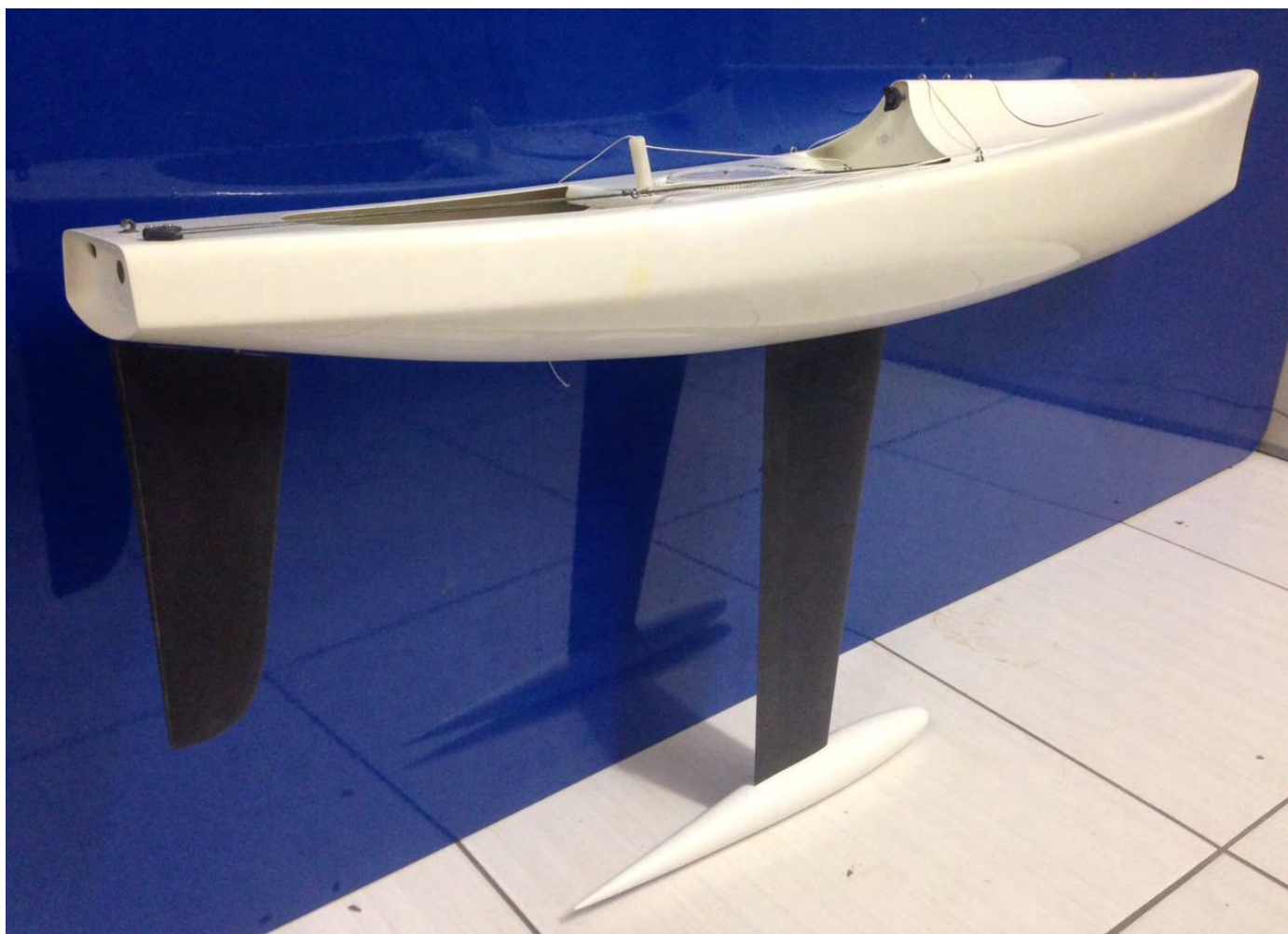
The Astbury fiberglass MERLOT. She is narrow with low wetted surface, and the waterline extends from transom to bow.
