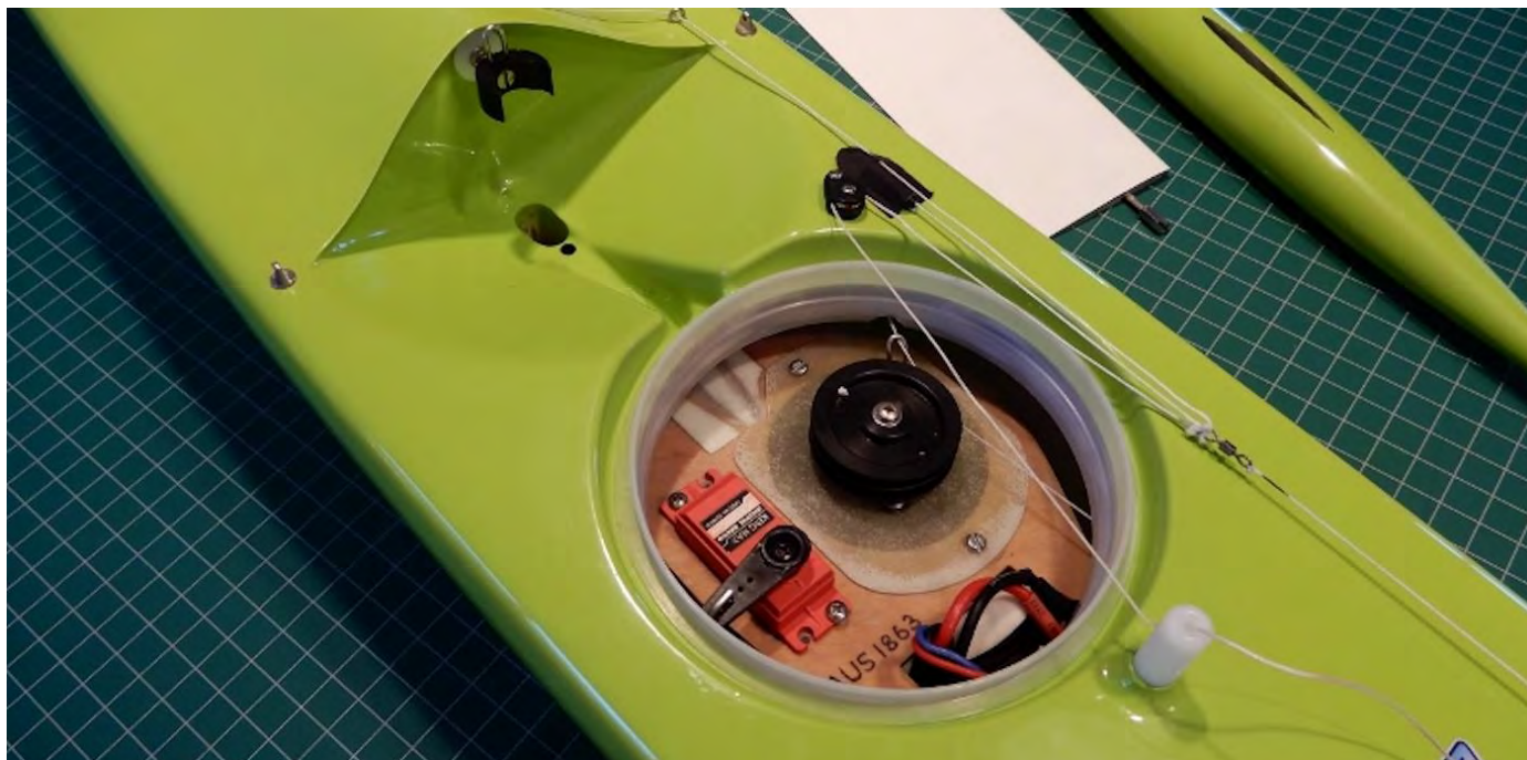
Tim's AKA proto showing the centralized electronics (plastic lid covers it). The production versions has no plywood.
