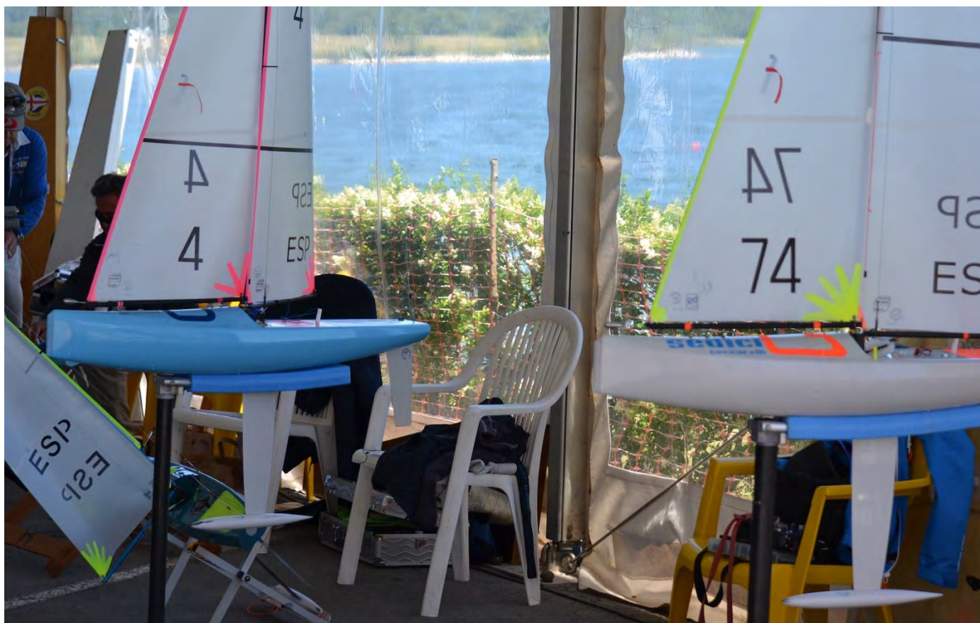
Two SIDICI designs from ESP at 2016 EUROS. Notice how the fin tapers to a shorter chord where it meets the bulb.
