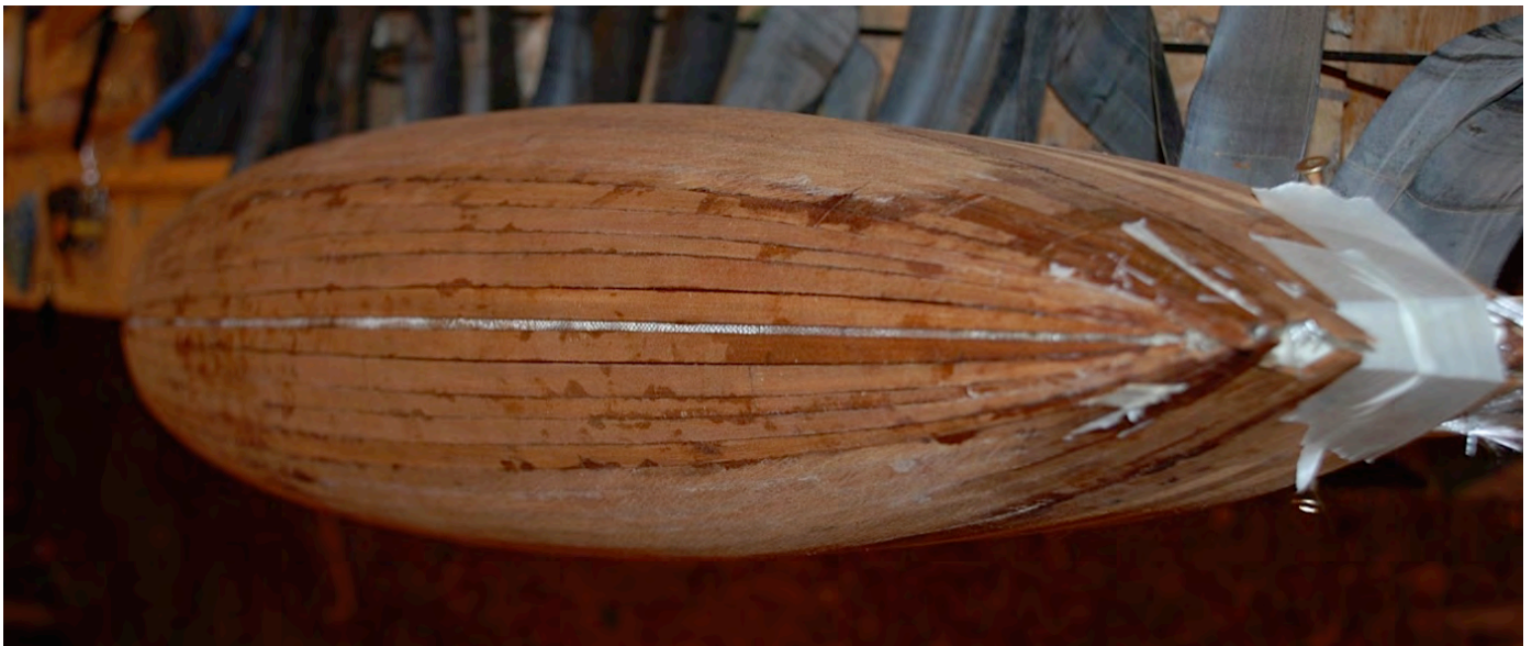
The hull planking finished and the sanding started.
