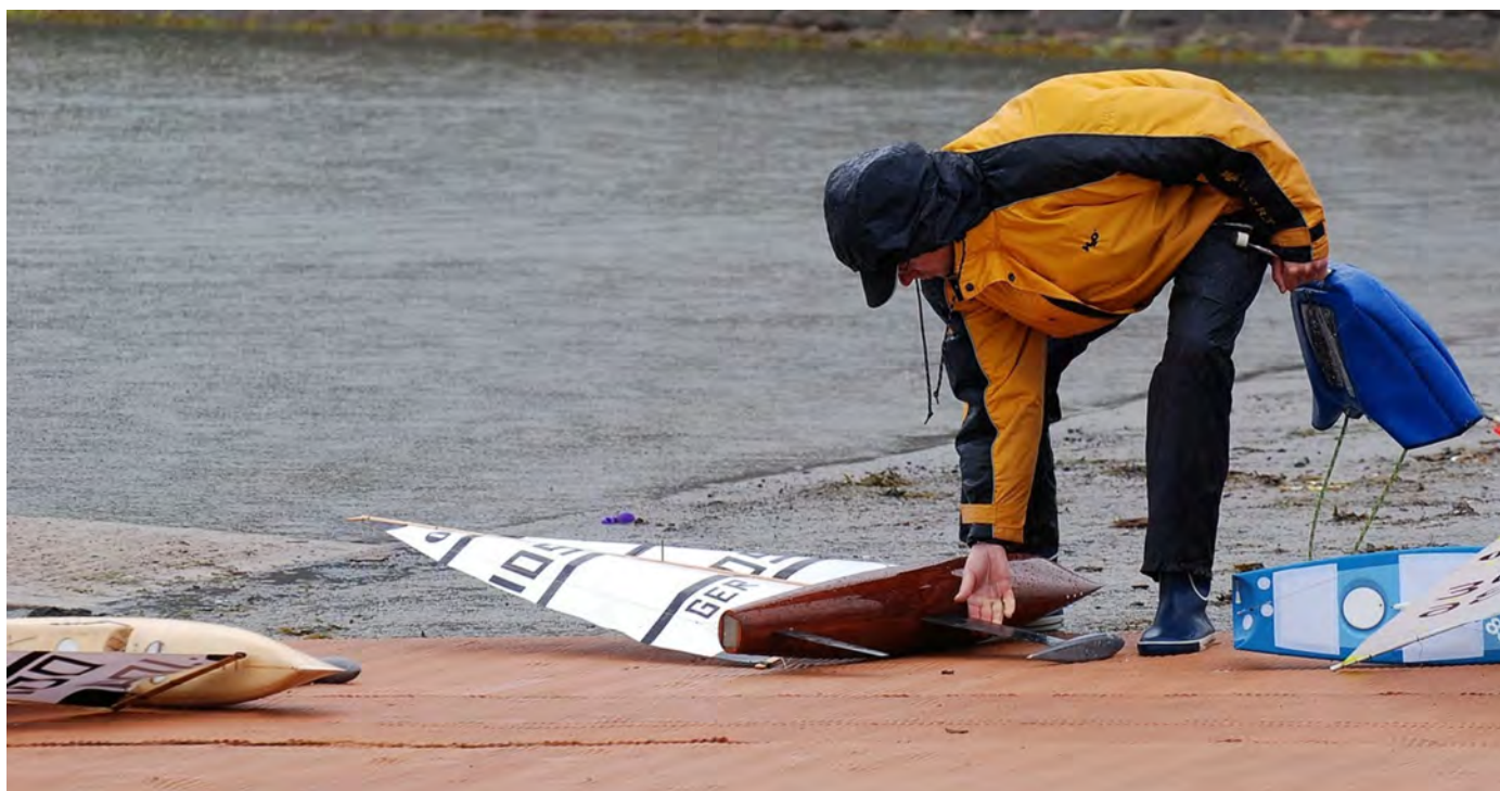
Michael Scharmer and one of his later pioneering narrow SCHARMINGS (center) at 2010 Worlds in West Kirby. Another German wood SCHARMING on the left shows the bow form. For comparison the PIKANTO on the right has a more conventional and much wider max beam for this period in IOM development. Hanneke Gillissen © photo.
