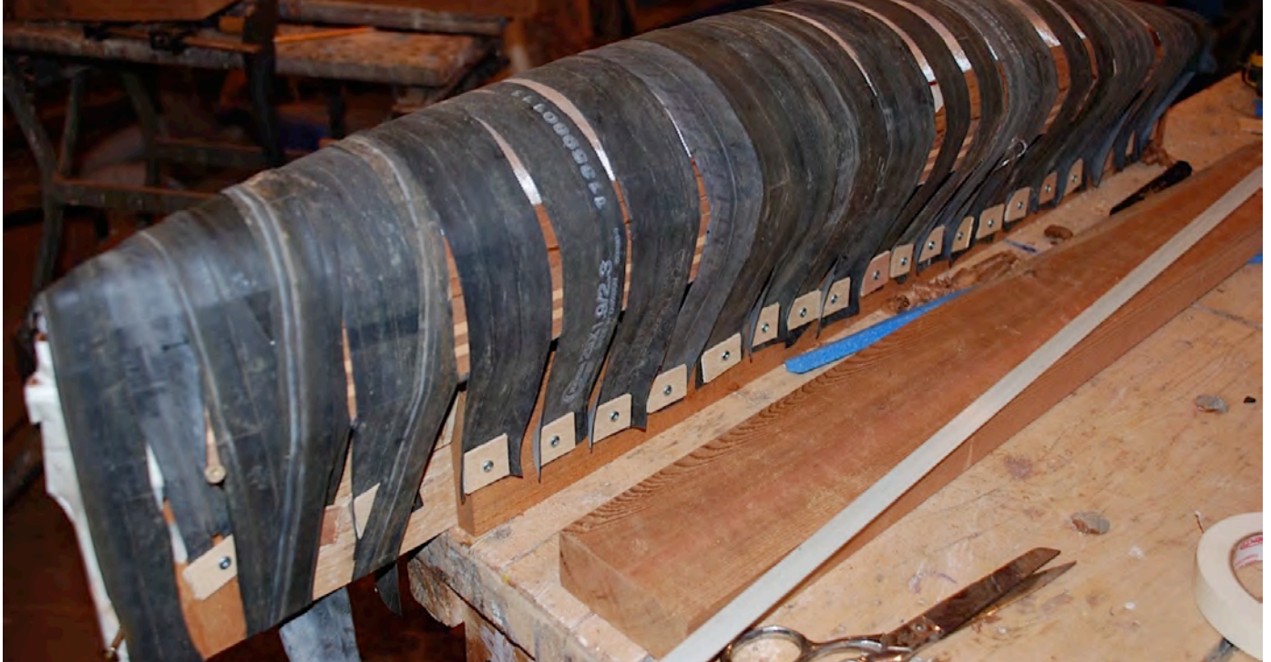
Here you can see the bicycle inner tubes holding the planks to the mould.
