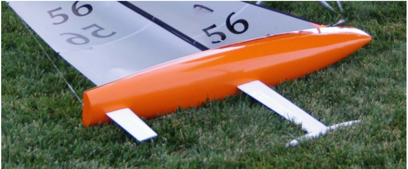
Jess Atkinson's Eldred V8 at the 2014 US Nats. I measured the rig tension on this boat and Ian Vickers' "Jumpin Jack Flash" at Foster City in August 2013. They were both very high at 14–15 lbs shrouds and 9-10 lbs backstay. Rig tension was high as I have ever measured on any IOM, and conditions were gusty in mid and upper 1-rig. Ian in particular was fast and smart, and Jess was... fast with very good sails. Thor Larsen © photo.
