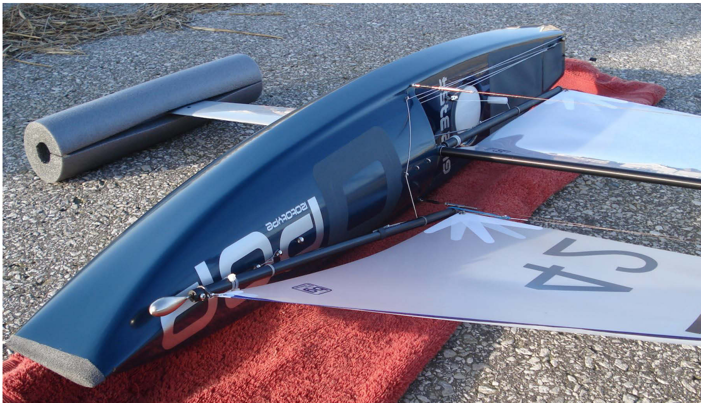
Another closer view of BG's POP. "Essentially the design is a fraction narrower overall, with a slightly raised bow to help alleviate any tendency to drop its nose downwind due to an overall bouyancy reduction." BG provided photo.
