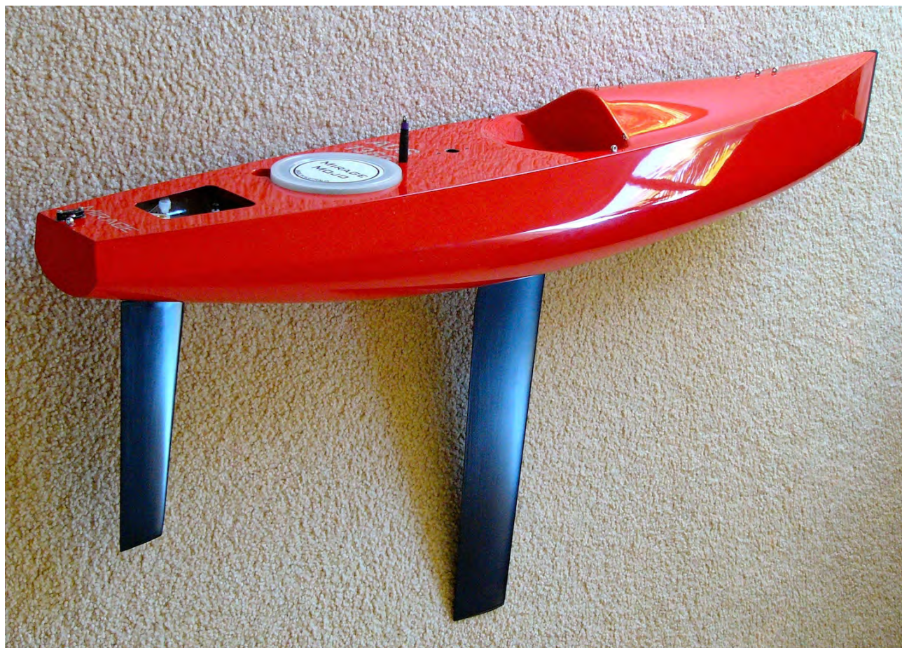
A view from the aft quarter of the new MOJO, and that is one long skinny (high aspect ratio) rudder. Photo Jeff Byerley.
