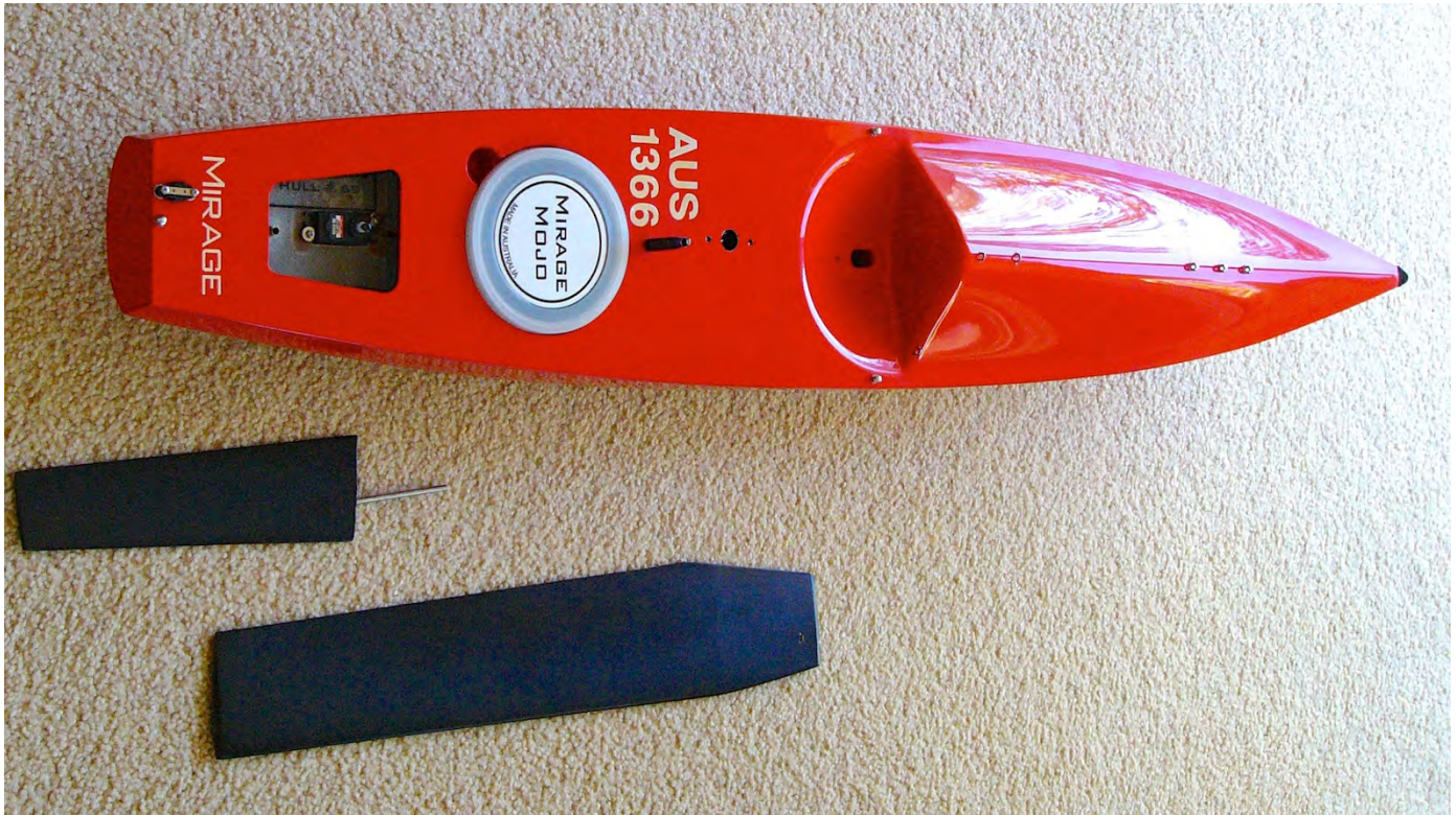
A view from above of the new MOJO, and you can see the rudder servo is placed well aft. Photo Jeff Byerley.
