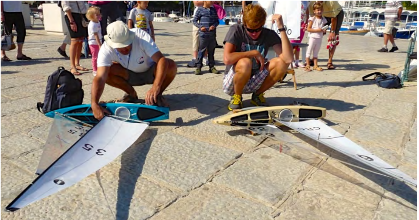
A visual comparison of the Kantun S (L) and original Kantun (R) in Opatija. On the Kantun (R) the deck openings are configured in a straightforward manner, but on Kantun S somebody stylized the openings until they were pointy at bow and stern. There is something to be said for both approaches, and both work fine visually. Duvancic photo.
