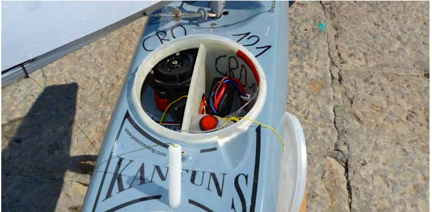
A view of the electronics container and lid is attached so it can't go far. Notice the deck depression providing a finger hole to lift the lid, one of the refinements added to the Kantun S. It appears very well executed. Duvancic photo.
