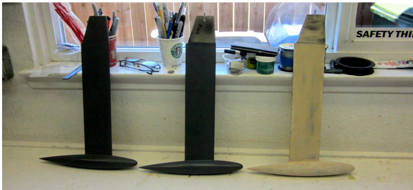
Some of Steve's MB-3 keel and bulb experiments. By this stage of development he was no longer trying the longer thinner bulbs. Steve Toschi photo.
