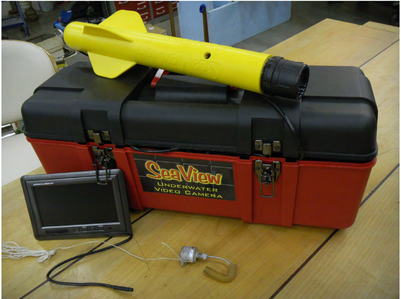
Proactive Deception Pass MYC's new camera for recovering boats in dark water, an investment of a bit under $1,000. Many of these are sold to crab fisherman to check their pots without pulling them up from the deep. The custom hook in front was on an 18" tether and the camera was used as a guide to hook the boat safely. Julian Lee photo.
