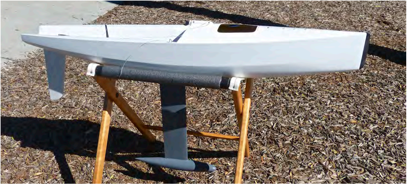
Steve's MB-4 at R6 in Foster City, which has a shorter and rounder bulb than a current Bantock or Creed. Topsides above the chine are vertical and the chine and deck edge are a sharp corner only slightly eased. Bob Wells photo.
