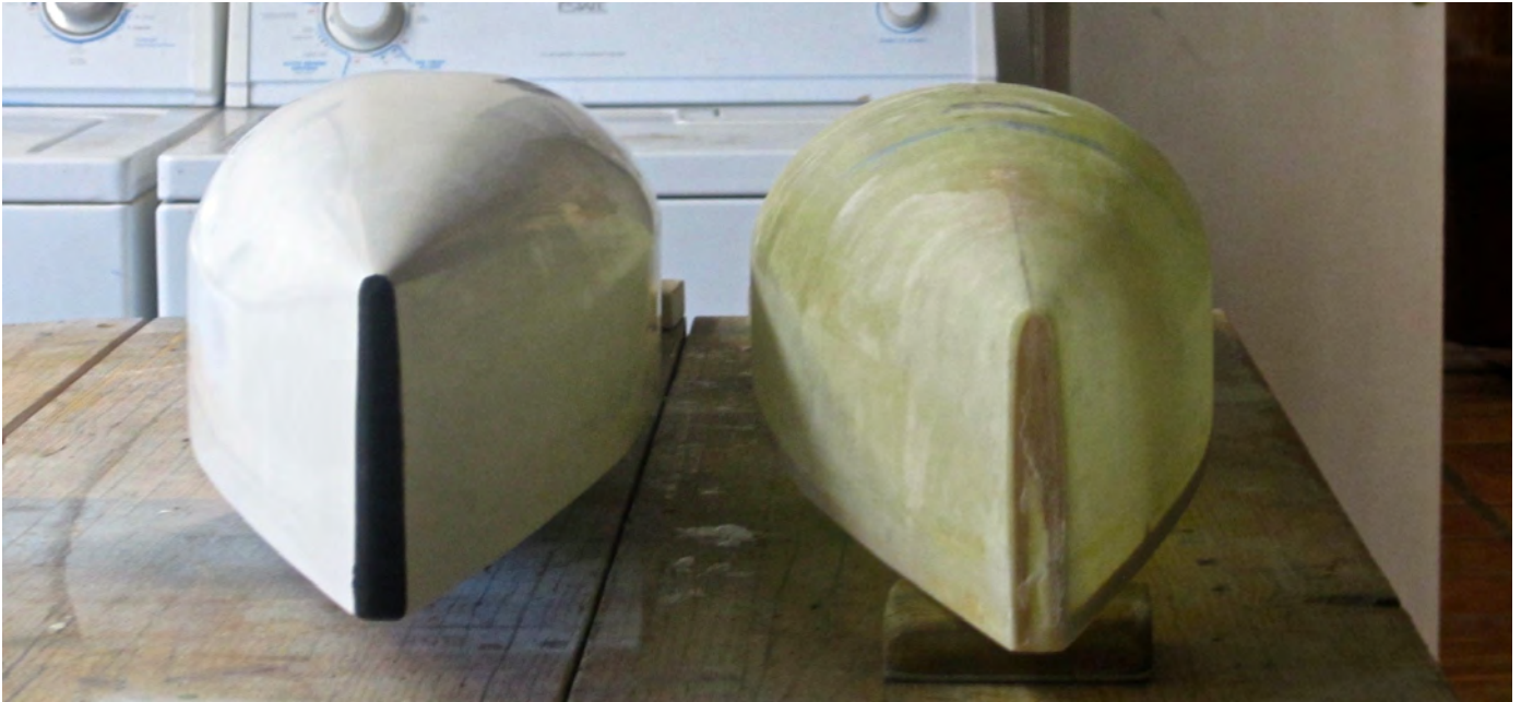
MB-3 is painted and MB-4 is unfinished. I can discern little difference other than a wider bumper on MB-4 allows a little more fullness forward. Steve Toschi photo.
