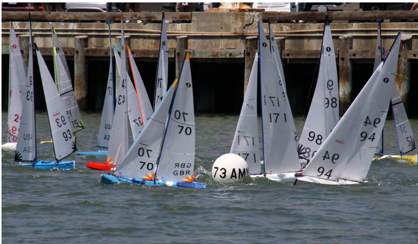
Far right is Steve Toschi's MB-3 #94 mixing it up at US Nats on San Francisco Bay. Notice he has a main leech telltale on his upper batten to indicate when over sheeted and/or vang'd. http://www.ellenhoke.com/
