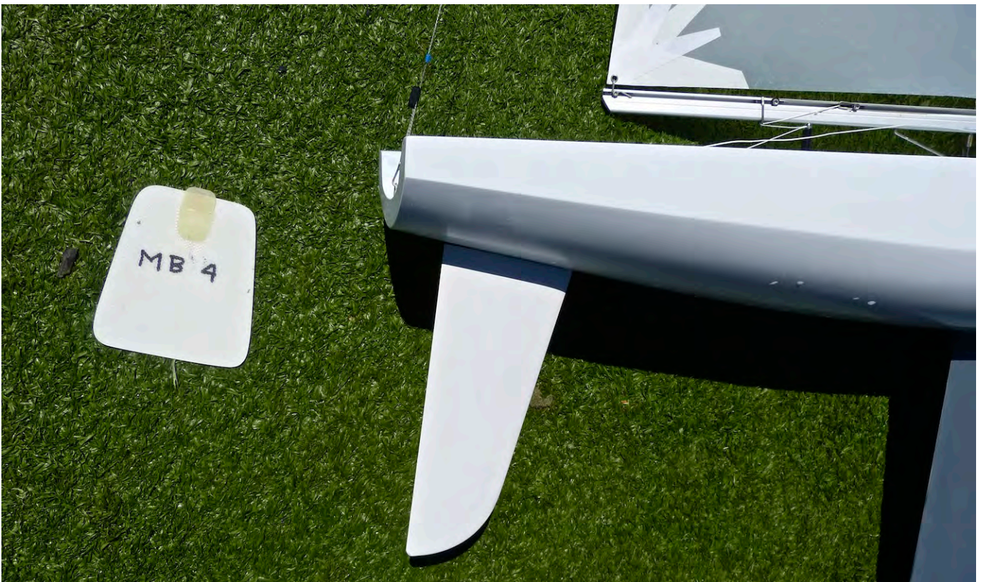
MB-4's rudder profile - note that it is moved well forward from the transom. Notice the foredeck hatch has a small tab forward, another nice little extra touch to lock it in place. Bob Wells photo.
