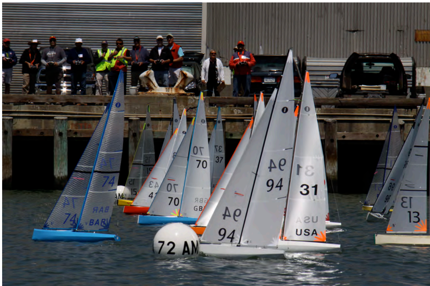
Steve Toschi's MB-3 #94 again at US Nats on San Francisco Bay, and this time in A-fleet. Notice the MB-3 chine arcs noticeably lower at mid-section than the Britpop boats #74, 70, and 31. Steve said, "The chine is located so that it is
