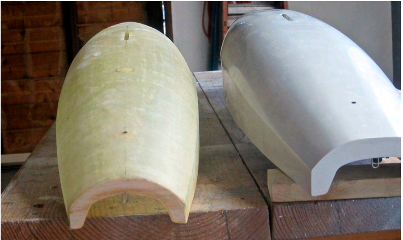
Differences are much more apparent at the aft sections. MB-3 (r) is painted and with segmented U-shaped sections. MB-4 is unfinished here and with much more rounded sections. Steve also said that MB-3 was a little thinner and had a lower aft deck, making it appear smaller aft. Steve Toschi photo.
