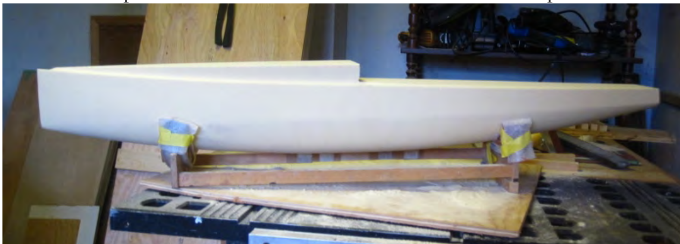
PP5 in raw CNC plug form before final foredeck shaping and surface smoothing. Note the low transom to reduce windage and weight in end. Photo David Cook.
