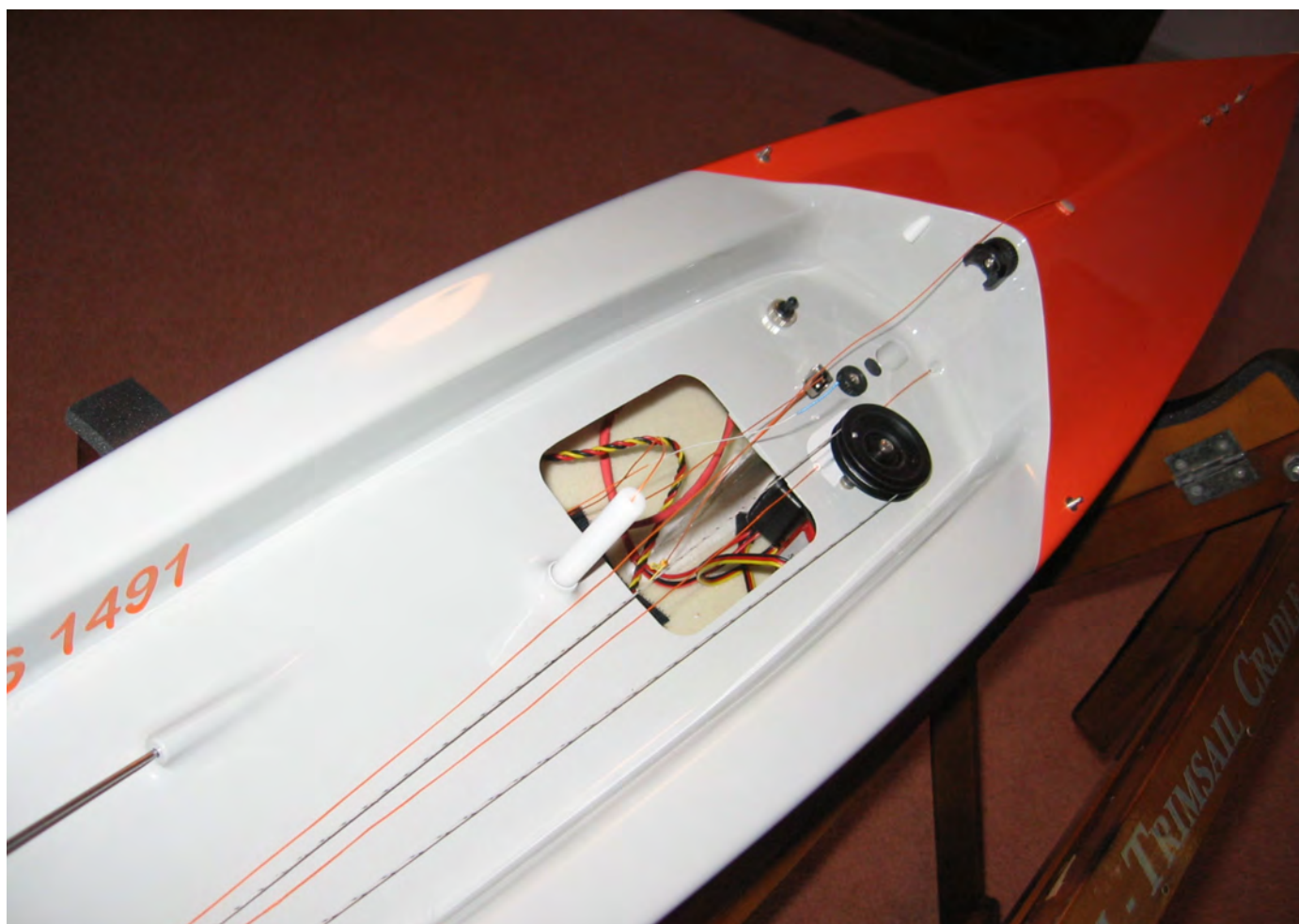
The Radio Race Yachts' PIKANTO showing the electronics in closer detail.. The rudder servo Futaba S3001. The pot for the battery fills the opening, see the previous PIKANTO image for that. The receiver is Futaba 6J. Elaine Brown photo.
