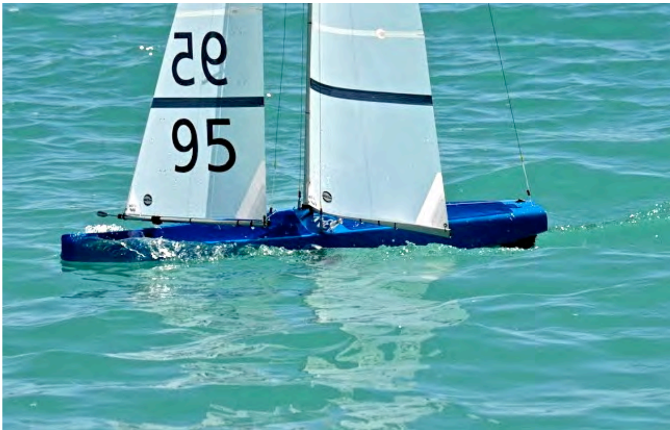
Graham Bantock sailing his FRAKTAL at the 2012 Malta IOM National Championship. Look closely and it appears that the bow knuckle is functioning well here to provide, "a clean break for water flow to exit from the hull". Hanneke Gillissen © photo.
