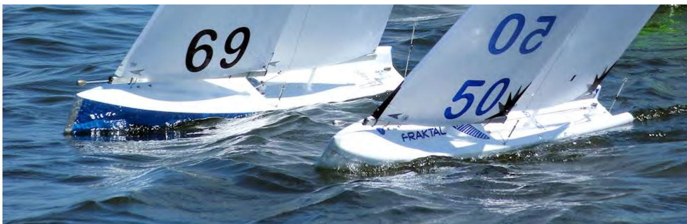
Radio Race Yachts skiff deck PIKANTO (L) and skiff deck FRAKTAL (R). The FRAKTAL has the noticeably fuller bow. Photo by Bruce Mathers.
