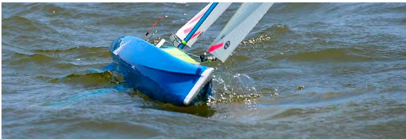
The distinctive reverse sheer and knuckle (or 'moustache' if you like) are pronounced in this SAILSetc built FRAKTAL owned by Peter Kampe. The foredeck patches are the giveaway that she is SAILSetc spec. Hanneke Gillissen © photo.
