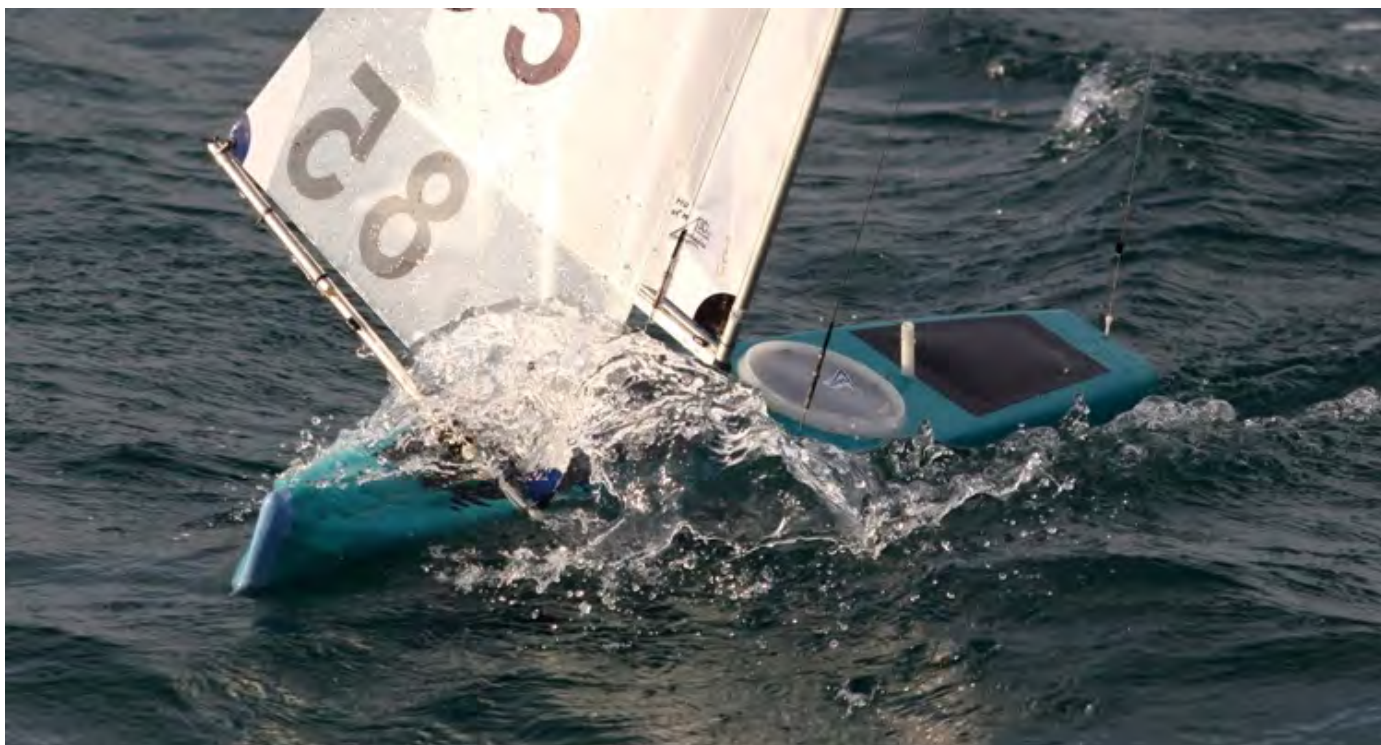
A Croatian flush deck FRAKTAL that was well sailed by Marko Matic to a top ten finish at 2012 Euros in Cres. It has since been sold, where it was described as molded by SAILSetc & finished by Zvonko Jelacic. SAILSetc offers FRAKTAL componts for assemble by owner. Note the plastic lid access to electronics, Zvonko's preferred access as seen on his new KANTUN's. Terrific action photo by Dean Miculinic.
