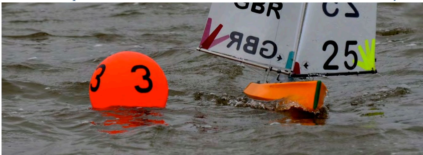
Rob Walsh's LINTEL MMX at the 2012 UK Nats – here showing her long chine, tumblehome, and flare at the foredeck edge. Hanneke Gillissen © photo.
