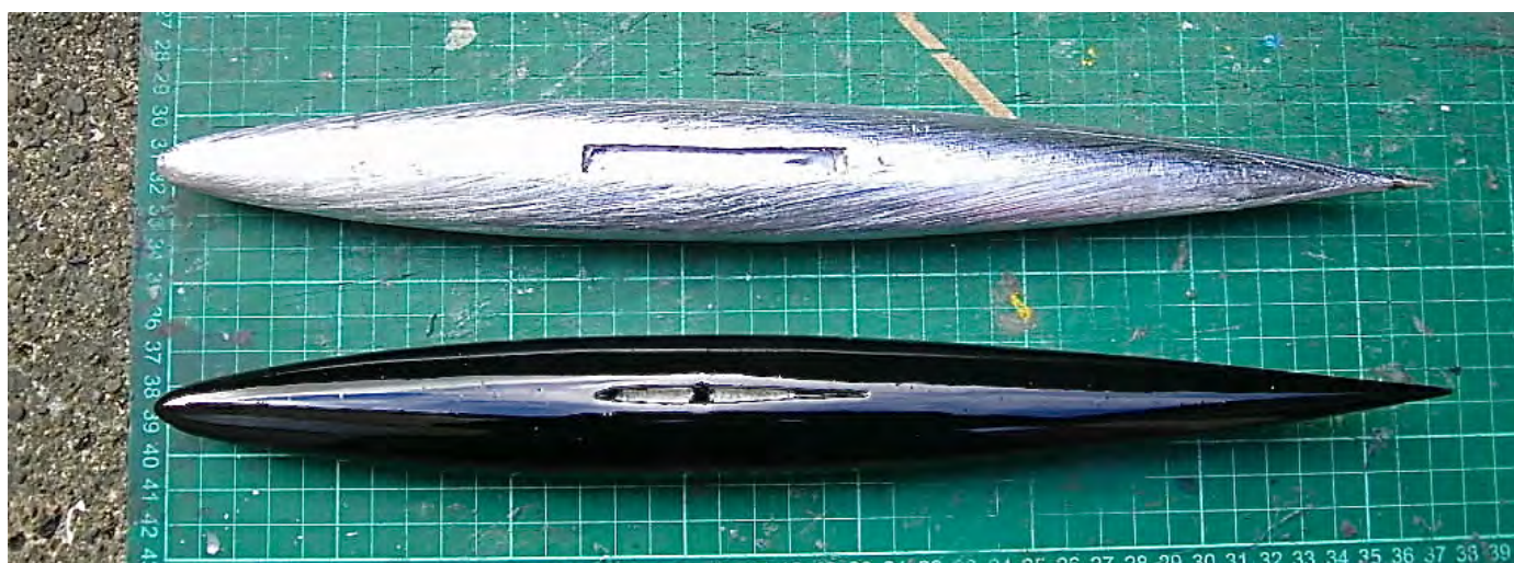
The Creed IOM bulbs before and after fitting the fin and finishing in the epoxy prime and two-pack finish coat. Dave has his reasons for preferring black, but some like me prefer a lighter color to better spot weed. Dave Creed photo.
