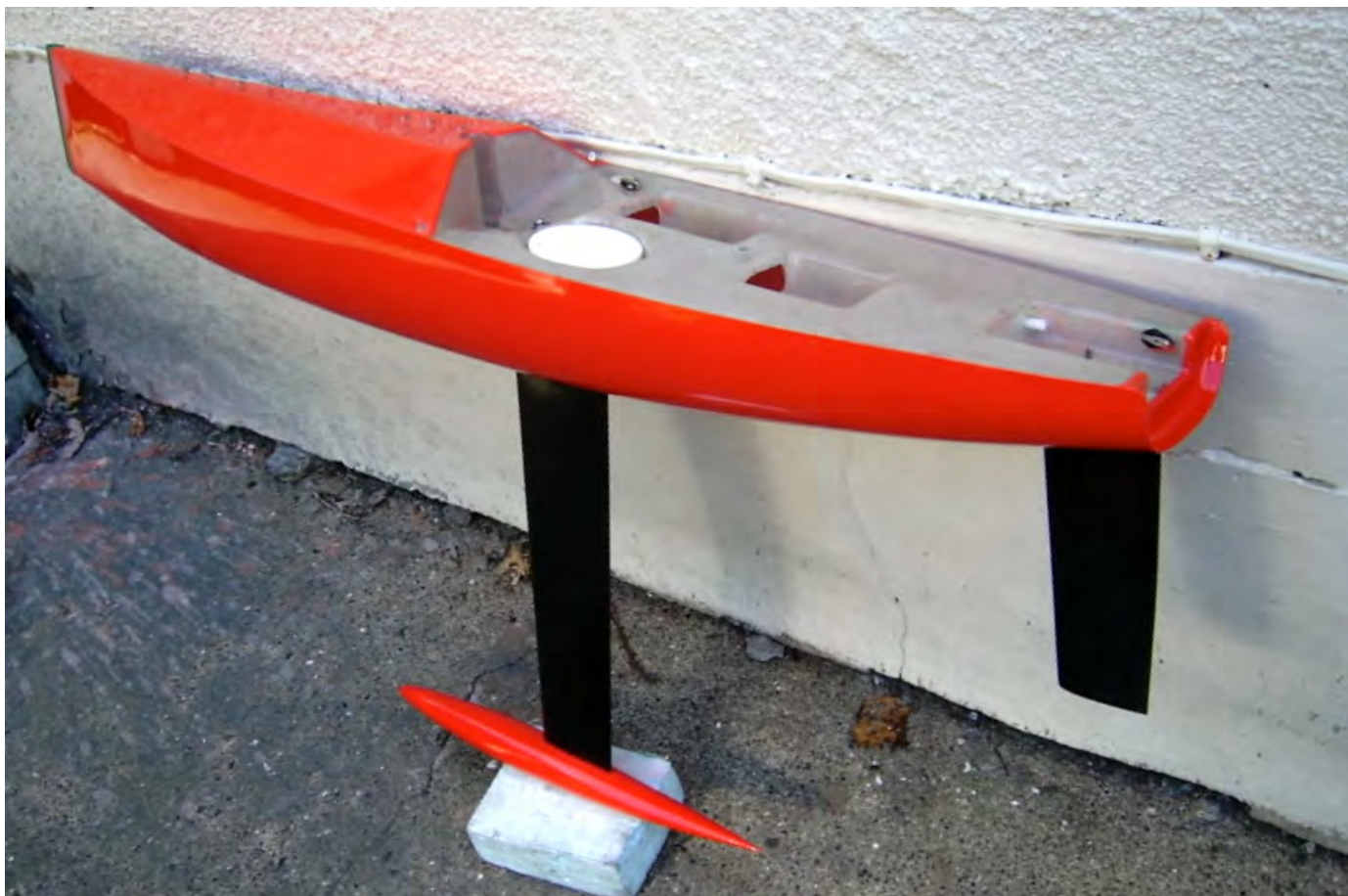
Martin Robert's VIPER #3, designed by Mark Dicks and built by Dave Creed – giveaways to who built this are the distinctive "universal" deck configuration that is in in clear resin finish to save weight. This boat finished 5th in the 2010 Euros establishing that in the right hands she certainly can perform. Dave Creed photo.
