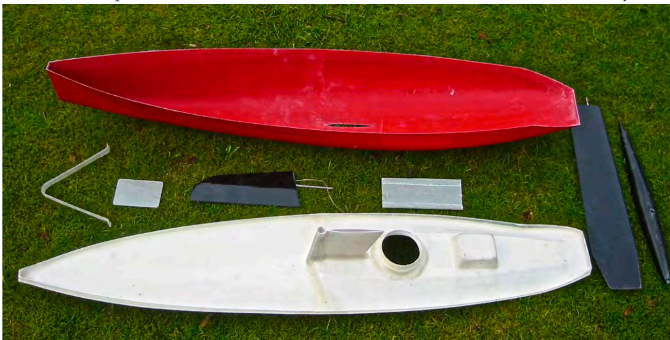
Creed Widget kit components. The special feature is the deck flange that aligns the hull and deck, including the critical fin/mast tube. This makes it all doable for an amateur homebuilder. Dave Creed photo.
