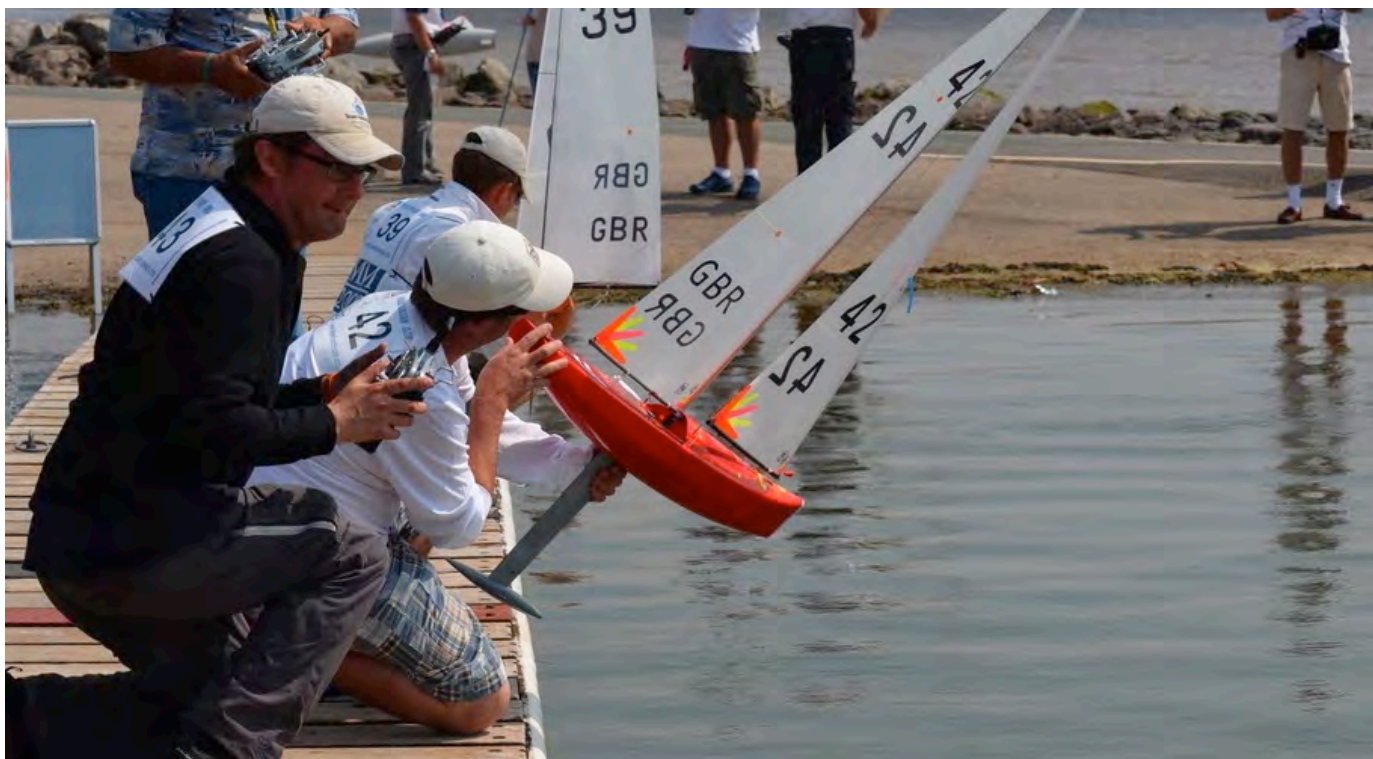
BG showing the technique to check his leach shapes at 2011 Worlds with Peter Stollery in the background. Base setting you want the leach twist parallel on both sails. Hanneke Gillissen © photo.
