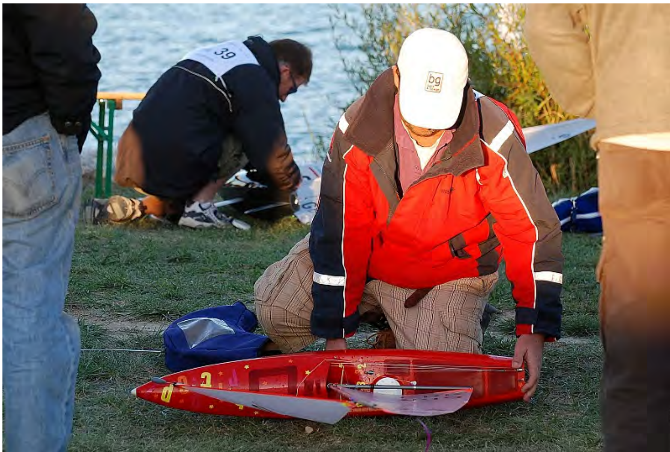
BG shown checking the BritPOP! prototype #1 trim at 2010 Euros, where he finished 2nd. Beam is atypically narrow compared to existing designs at that time, the exception being Michael Scharmer's series of ultra skinny designs. Sail trim shows an upper batten aligned with boom and the outhaul is pretty flat too. Hanneke Gillissen © photo.
