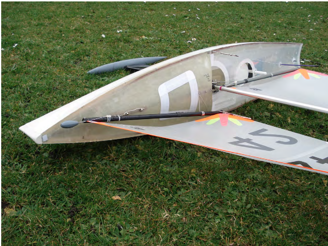
A late SKA proto that was part of the development of Britpop – photo date 3/24/10. This shows the flush deck skirt experiment similar to the ones BG used on the Disco at Vancouver 2003 Worlds. Brad Gibson photo.
