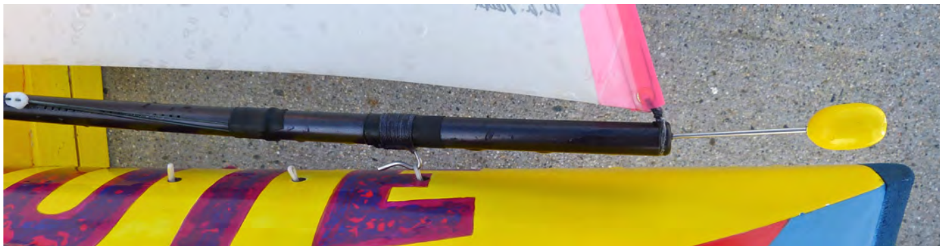
Jib swivel is a stainless hook lashed and glued to the boom. Each rig swivels on its individual string in an individual tube that extends to the hull bottom. Bob Wells photo.
