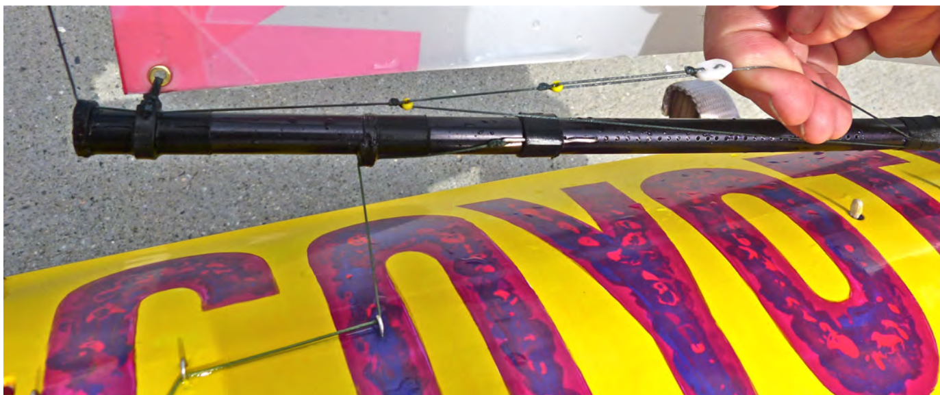
Jib boom is a Easton 7/16" tent pole with 4-part topping lift for fine-tuning located along the boom for less windage. Bob Wells photo.
