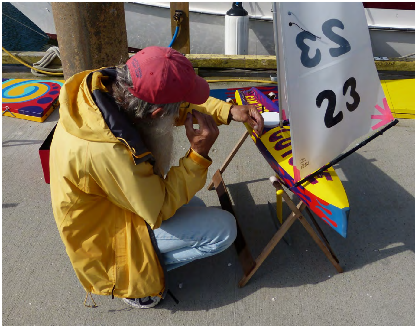
Graham Herbert adjusting his custom COYOTE's shroud tension at Saltspring Island Sailing Club, which is silly easy with his system. The hull form is another new boat inspired by Brad Gibson's BritPOP! The hull graphics extend to the sail box seen beyond the transom. Bob Wells photo.
