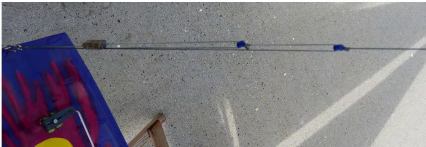
Backstay with 4-1 purchase for fine-tuning uses glass beads. The tiller arm and bowsie are custom made of course too. Bob Wells photo.
