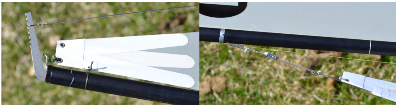
Details of Ian's A-rig. It's simple with no luff jackline and a sizeable gap at mainsail and mast. Photo Jerry Brower.
