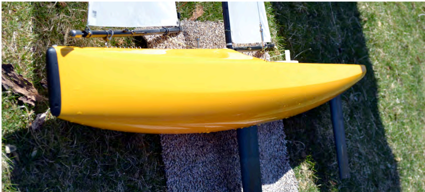
A hull view showing the rounded sections, the rocker profile, and the chine. Jerry Brower photo.
