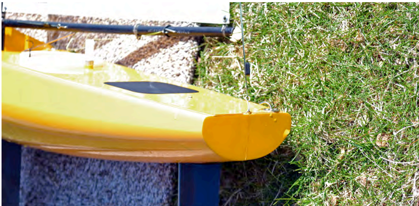
The transom and a flush deck aft of the mast, which is a change from the V5 – V7 designs. Jerry Brower photo.
