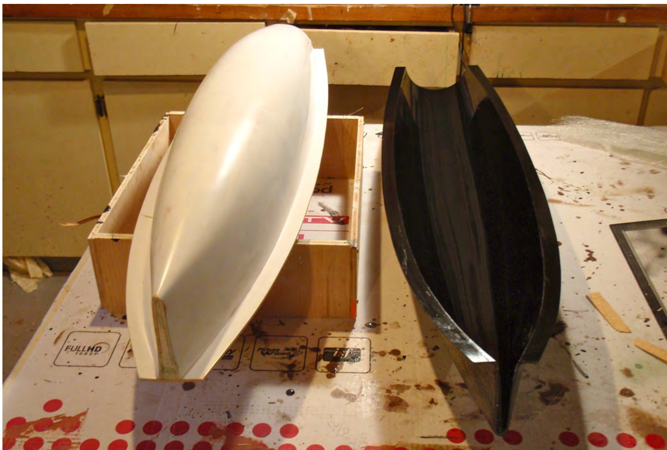
The plug is on the left with the hull mold just removed from it. The PVA has been washed from the plug.
