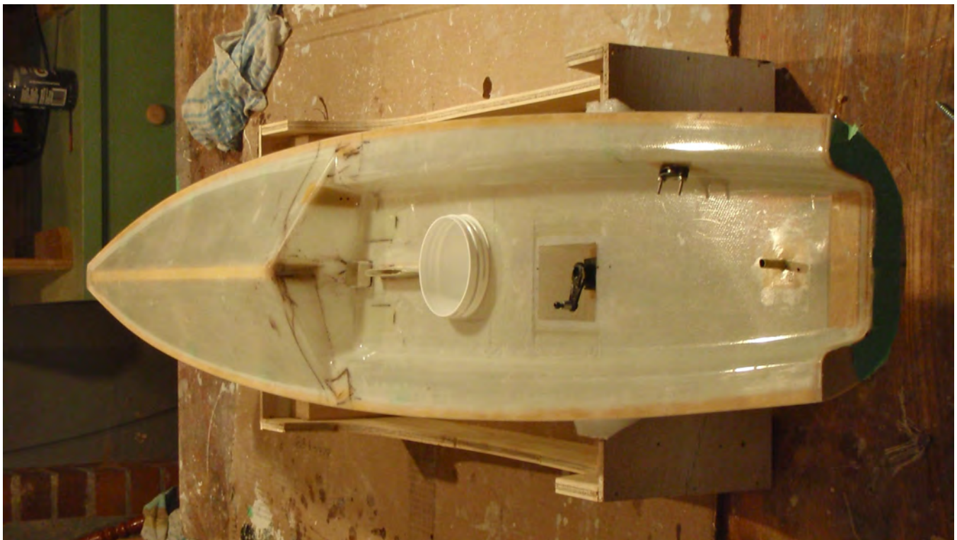
I asked Adrian how he joined his hull and deck: "The gunwales are 6mm strips of spruce or yellow cedar, whichever I have handy at the time. A good coating of thickened epoxy is smeared along the top of these and then the deck is centered and taped down all along the edges. Most of the deck flange is trimmed off using a Dremel tool before gluing; I only leave about 4 mm to play with. After the epoxy has set up and the masking tape removed I use 25mm wide sandpaper files to finish the job off. It's a good idea to put a few strips of masking tape along the hull near the sheer line when you do this so you don't accidentally scratch the hull. Done carefully you will end up with a perfect sheer line. Centering the deck on the hull is relatively easy, because I have centering marks built into the deck mould which of course transfer onto the deck at bow and stern." Adrian Harrison photo.
