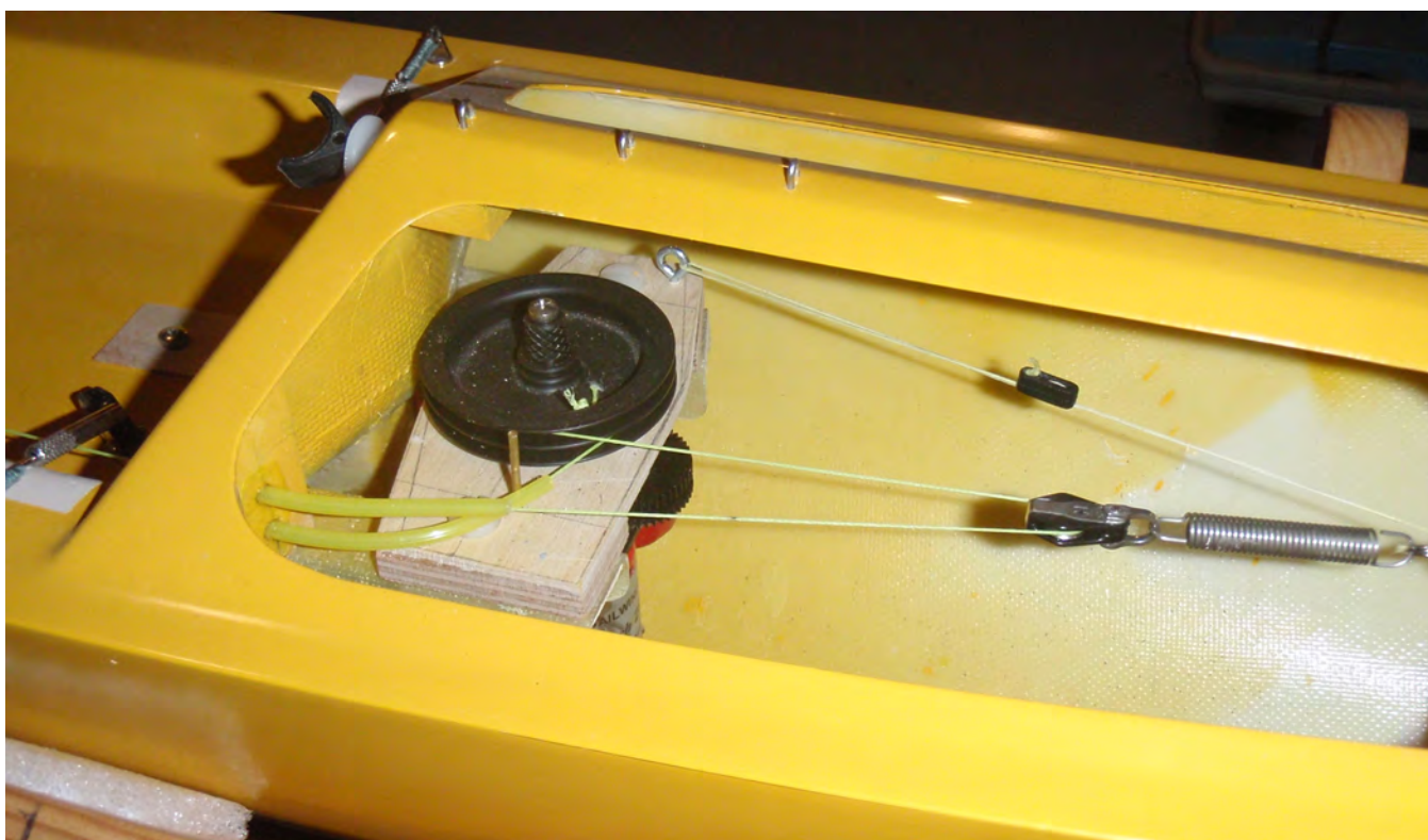
This SKA is the Dragon Lady, #2 out of the moulds. The RMG installation is shown with the special care to have the sheet and return lines running fair for no overrides. Simple, clean, and easy to maintain. The RMG winch is placed forward of the mast as I see on all BG boats. Photo Adrian Harrison.
