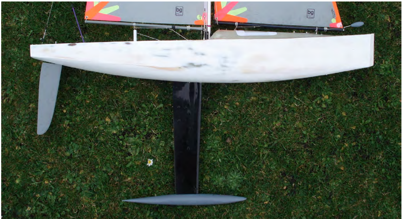
BG's SKA prototype: Mk12 Reggae mod trialling chines. Note rocker profile change aft of fin from Mk1. Using Eldred rudder as the improved maneuverability with added volume in the ends no longer required the large rudder. Brad Gibson photo.
