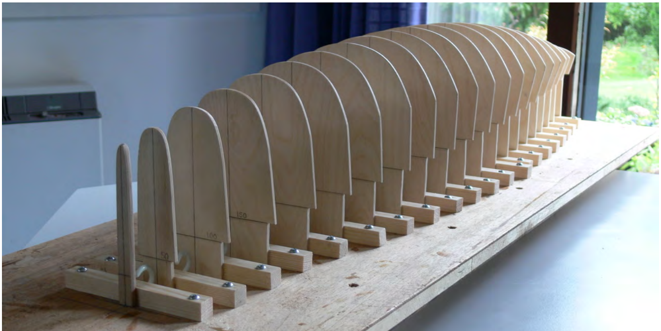
The shadows for Ian's wooden hull #4, CORBIE, show a very different hull form that Jeff Byerley describes more fully below. I'll remind you that this is a variant of the production Cheinz design by Mirage Radio Yachts, and not a reproduction in wood. Ian Dundas photo.
