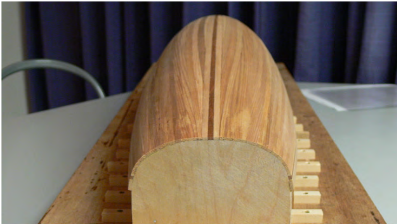
Ian's wood hull #3, ECO, showing a more rounded transom profile without chines. Ian Dundas photo.
