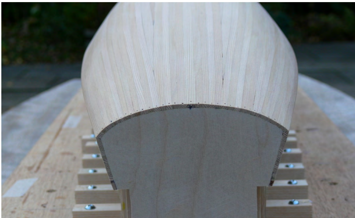
Now compare Ian's wooden hull #4, CORBIE's flatter bottomed transom with chines and tumble home. This is an early look at Ian's unfinished CHEINZ variant in wood. Ian Dundas photo.
