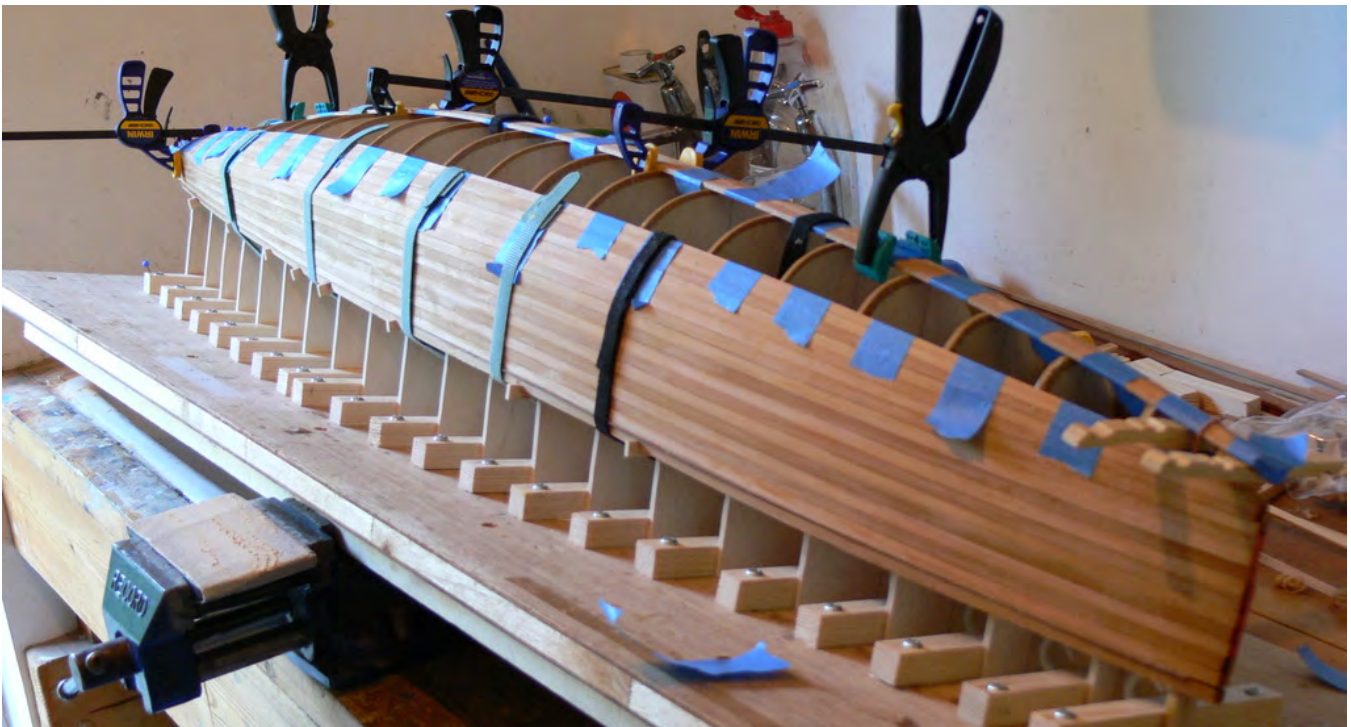
Now compare Ian's wooden hull #4, CORBIE, during planking. This is an early look at his unfinished Cheinz variant in wood. Both #3 and #4 are Mirage Radio Yachts designs, but are very different in hull shape. Ian Dundas photo.
