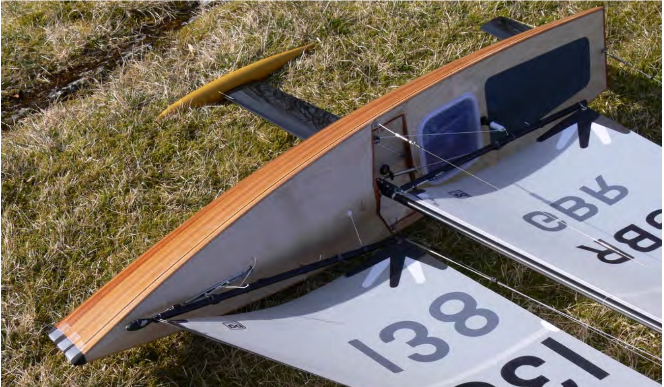
Notice the very clean plywood foredeck. Ian has adjustable eyes in a recessed track for his jib swivels.
