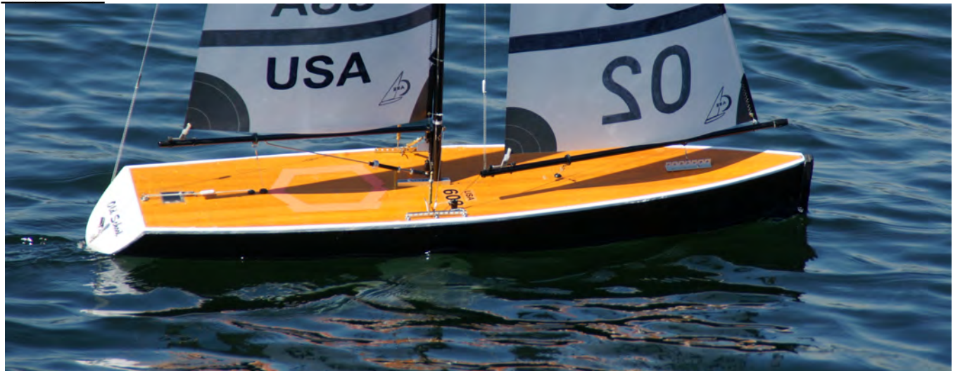
Rod Carr's "sweat equity" Zoom Old School sports a plywood flush deck. How different this Zoom looks from those with skiff decks as built by the Herbert brothers. Photo Ron Hornung.
