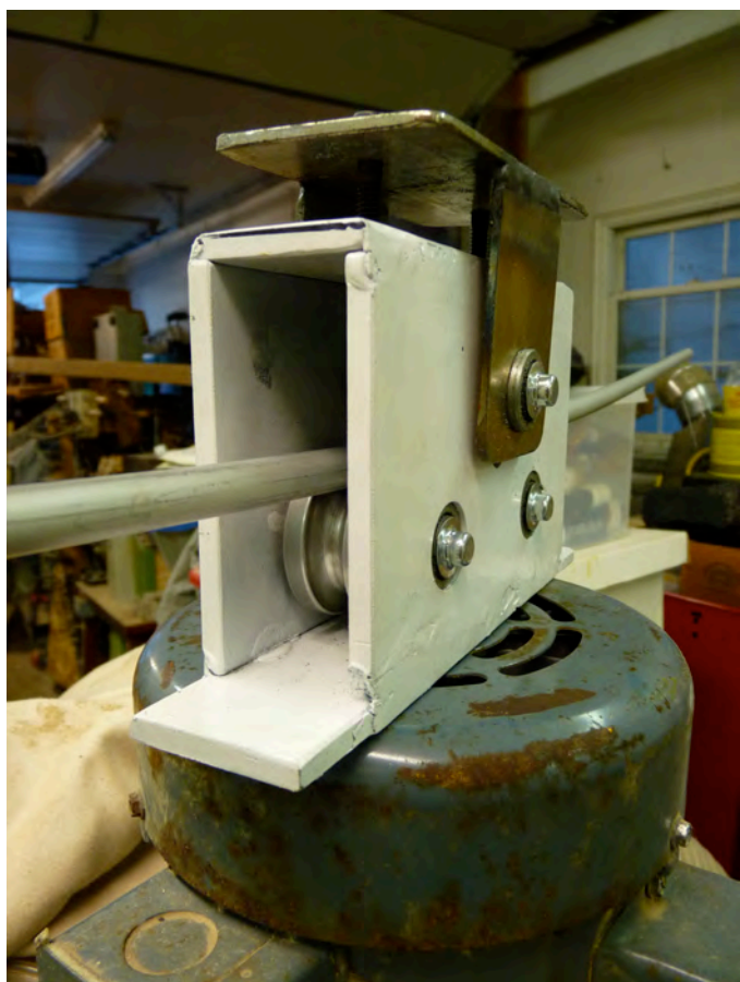
Bruce Anderson's custom prebend tool shown with prebending in progress. Bob Wells photo.
