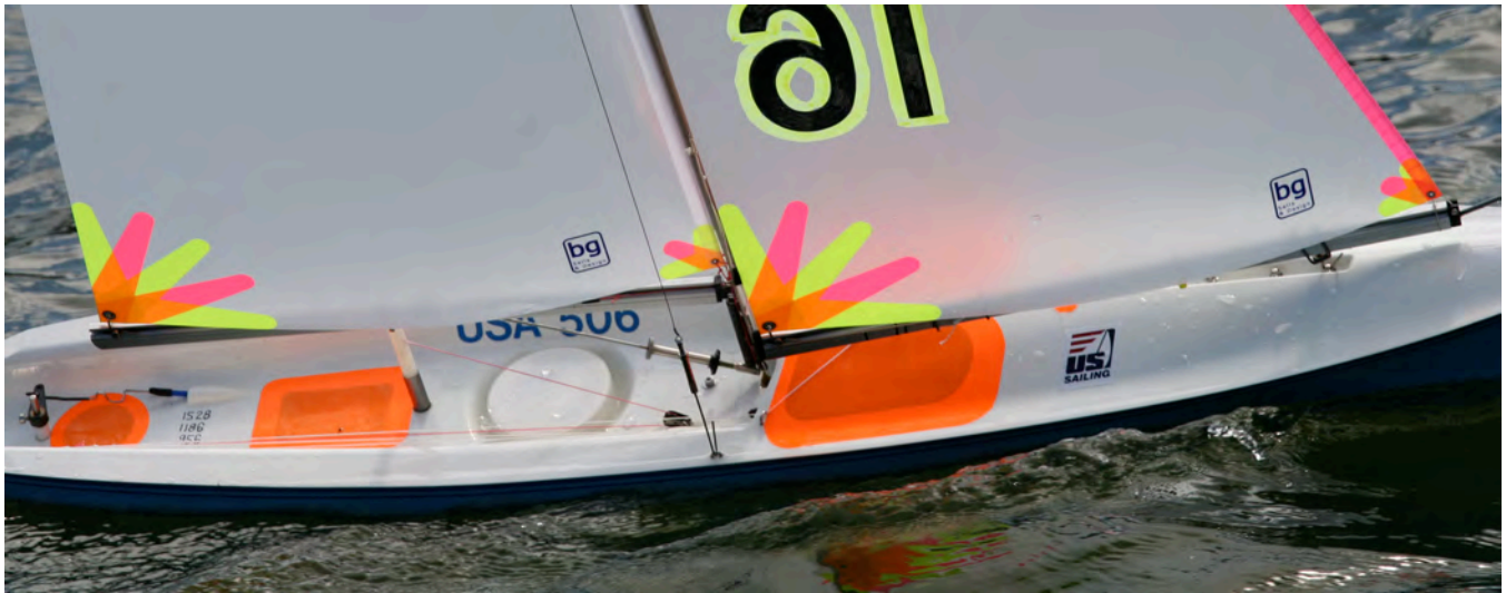
Bruce Anderson's Widget at Hood River Carnage, complete with colorful sails and deck patches. Note that his "base" rake setting numbers for each rig are shown on deck. No looking in the toolbox required. In this case rake is measured from aft deck to masthead, and I believe he got these from either the boat manufacturer (Elliot Yachts) or sailmaker? – Photo Ron Blackledge
