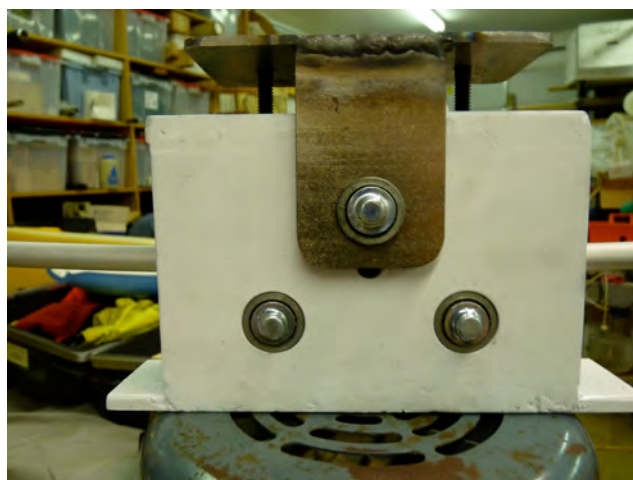
Side View of Bruce's custom prebending tool.
