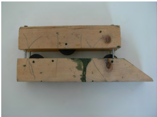
Ian Dundas' three-roll bender from more humble materials. Ian Dundas photo.
