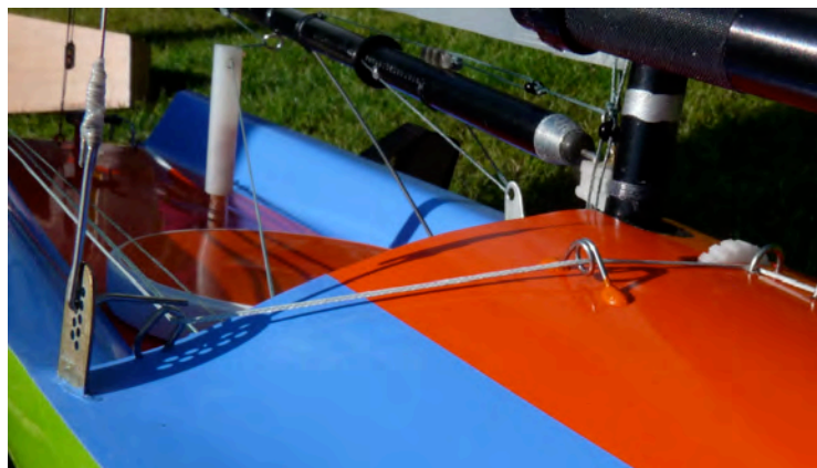
Shroud termination via hook and tang with narrowly spaced adjustment holes instead of a turnbuckle. This is Julian Laffin's Zoom from Hornby Island, built under the tutelage of designer Graham Herbert. Bob Wells photo.
