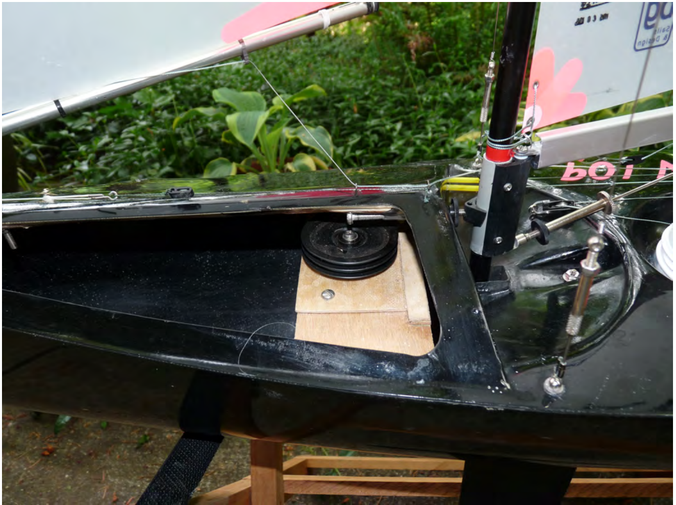
Porky Pig's details around the mast area with the winch forward of the mast. Bob Wells Photo
