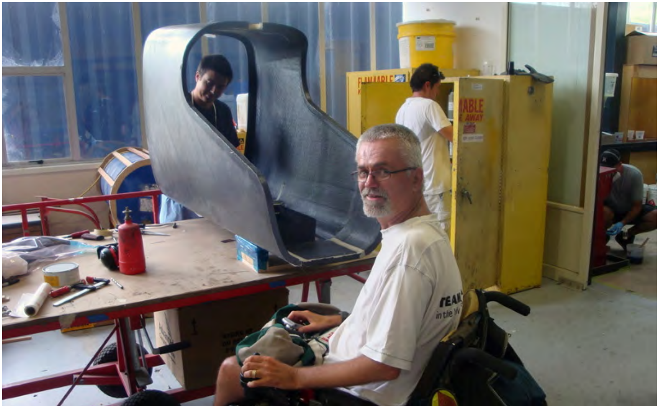
David with a carbon AC45 transom moulding at Core Builders Composites in NZL. Keith Taylor photo.
