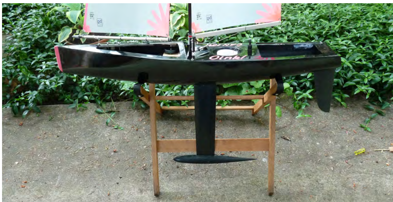
David's first build, HAMF BECK DOG, had a skiff type aft deck. Porky Pig has a flush deck aft of the mast with a well for the boom vang keeping the rig low, which is similar to Graham Bantock's designs. Bob Wells Photo
