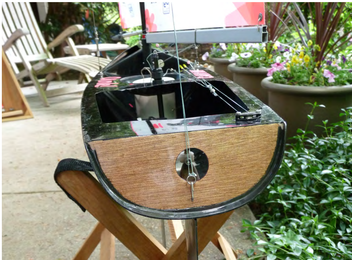
Porky Pig's mahogany plywood transom with a hole for rudder access that is covered with a patch when sailing. Although chines are all the rage now in IOMs, David is designing for light-medium air so he chose to avoid them in favor of less wetted surface. Bob Wells photo.
