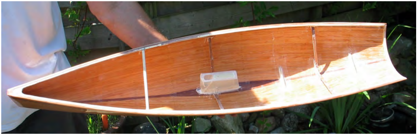
The hull looks nearly ready to receive the deck. Photo © Hanneke Gillissen.
