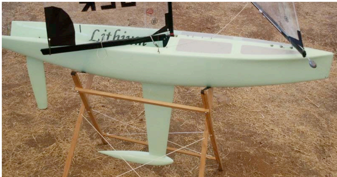
A much older sister: This Scharming finished 4th in the '04 Euros in ESP, and is a painted example of his earlier skinny chine hulls in plywood. The foils and bulb have evolved considerably, but the hulls appear to be a more incremental progression with a consistent narrow beam. This photo is from Anders Wallin's web site.
