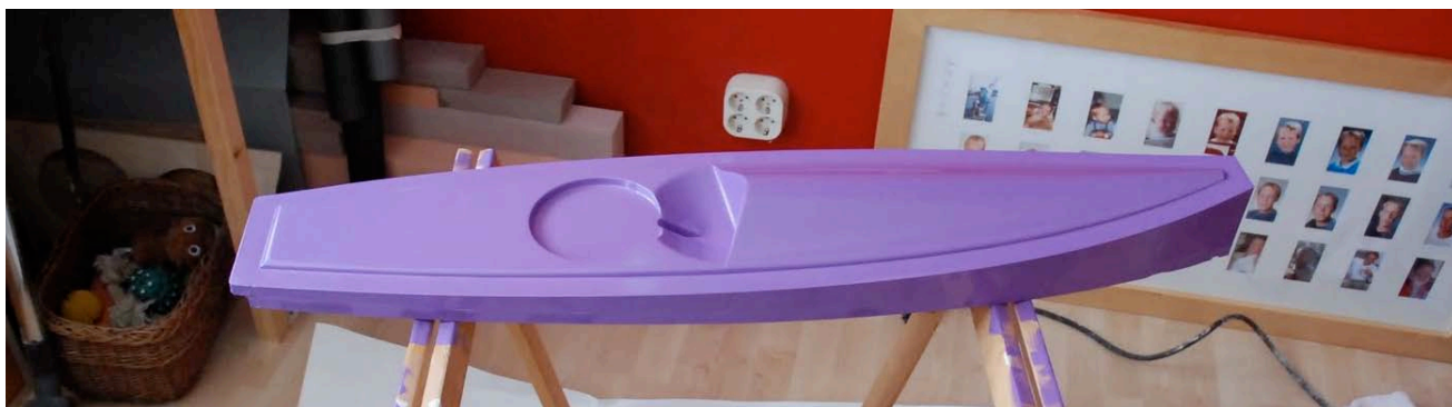
The deck plug with flange for Ace from the NED with a flush aft deck. Photo © Hanneke Gillissen.
