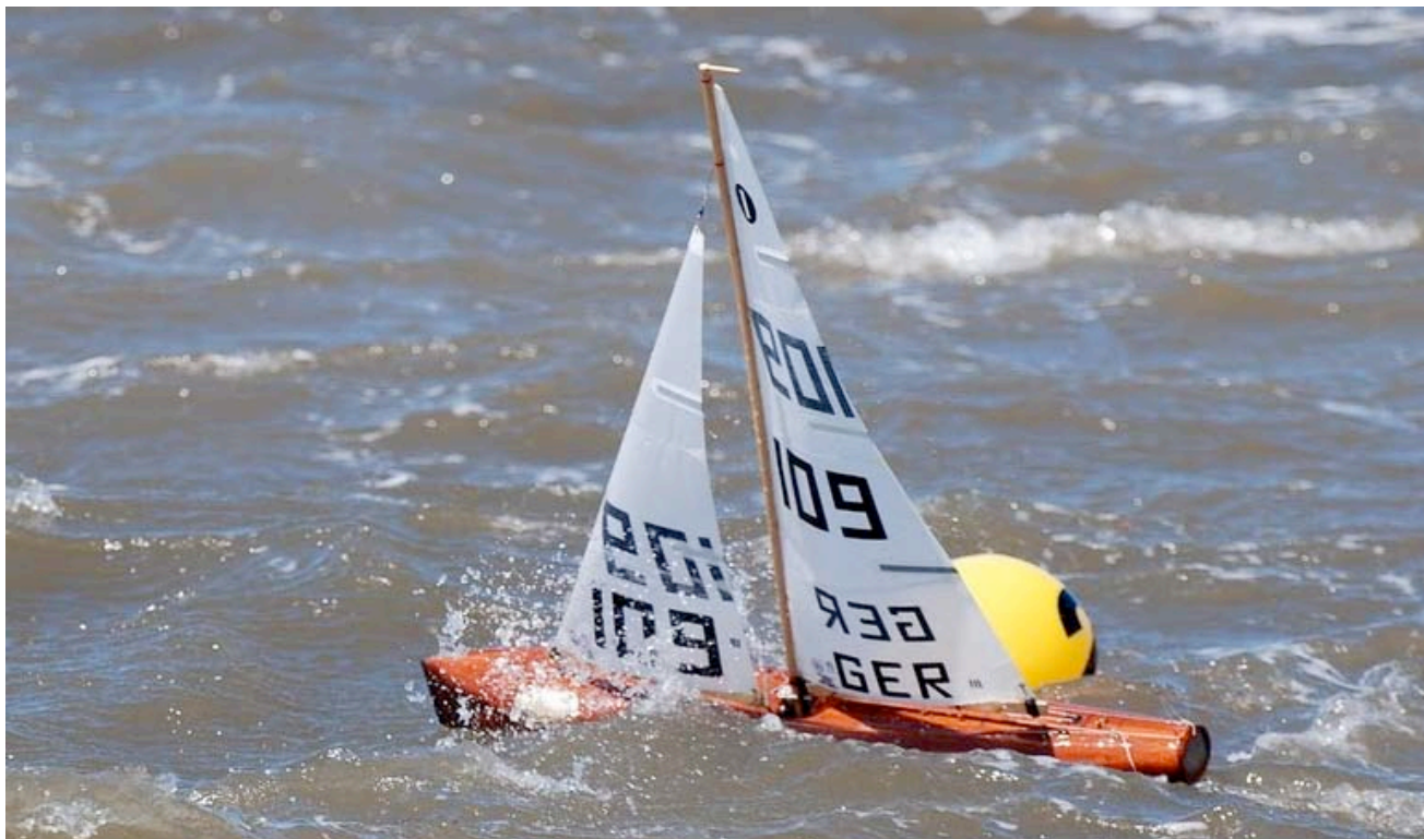
Scharming Mark-XVc at the 2010 GBR Nats in brown turbulent W. Kirby waters – note the aft bend in the middle-upper portion of the mast. I'll speculate that this inverse bend is caused by pounding in waves coupled with that flexible mast. This is not good of course. Among other things it allows the jib luff sag. Photo © Hanneke Gillissen.
