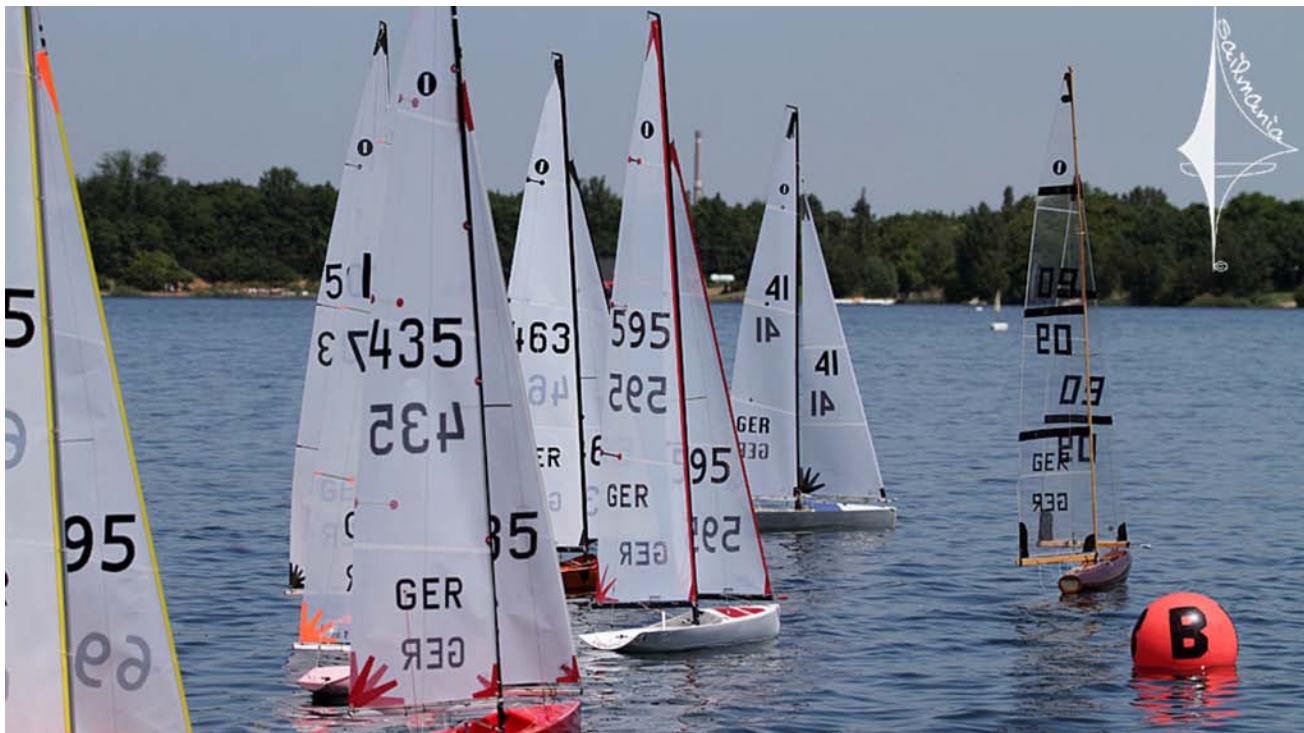
GER 09, a Scharming Mark XVc on the right. I included this photo to illustrate how skinny this design is. The A-rig sails are from Cellophane fabric, supposedly from a florist? It appears Michael makes his sails. Photo © Ingrid Bluem
