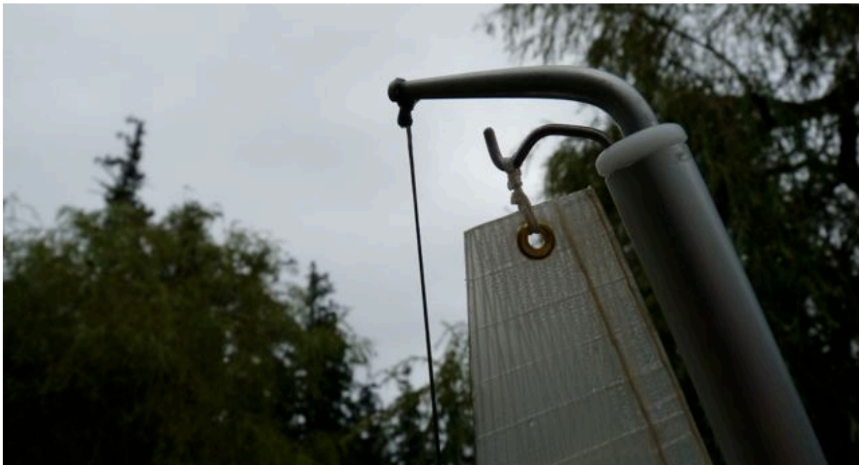
Graham's masthead has a tapered crane. It is all pretty conventional, just not the commercially available fittings most of us use. Note the gap between mast and main luff.
