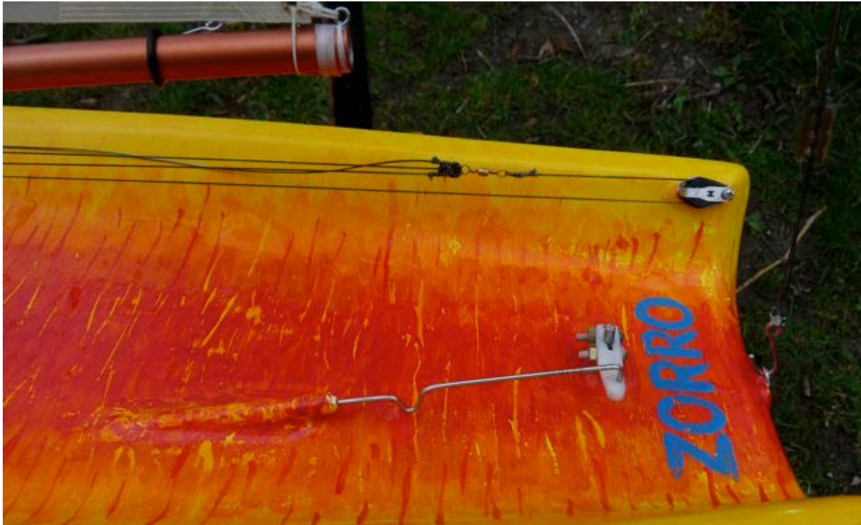
The bend in the rudder push rod allows fine-tuning the length?
