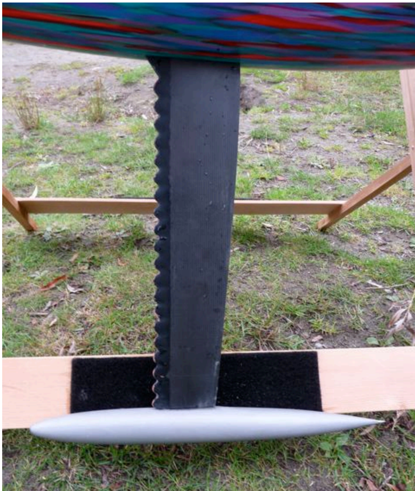
Graham Herbert's – fin in larger scale. Graham makes his own foils and bulbs, and is obviously an experimenter. This bulb is a longer one than usual for him. He now thinks he prefers the shorter/fatter one.
