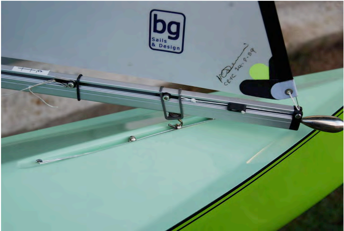
BGs "Arrival". This is a 2-rig, but note the string in the groove. I'm sure this is part of the A-rig string swivel, with the view blocked by the boom. Standard SailsEtc boom and fittings used on this boom. Note how low the boom is though. I imagine the groove adds deck stiffness as well as lowering the boom a few more millimeters.
