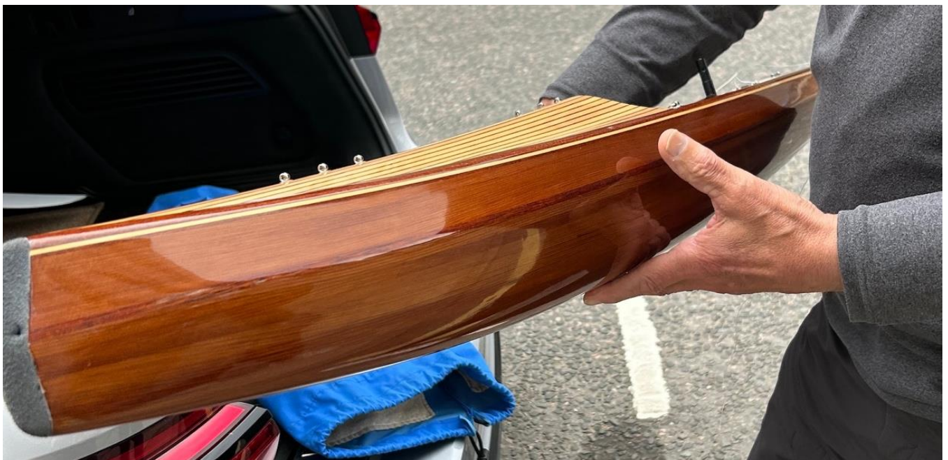
Ian's new design again, with a sapwood cedar hull, but this time with mahogany used at the chine and hull-deck joint to increase durability. In my few days in Scotland the wind blows all the time, so collisions there could have some force. Much more force than my light wind Seattle area.
