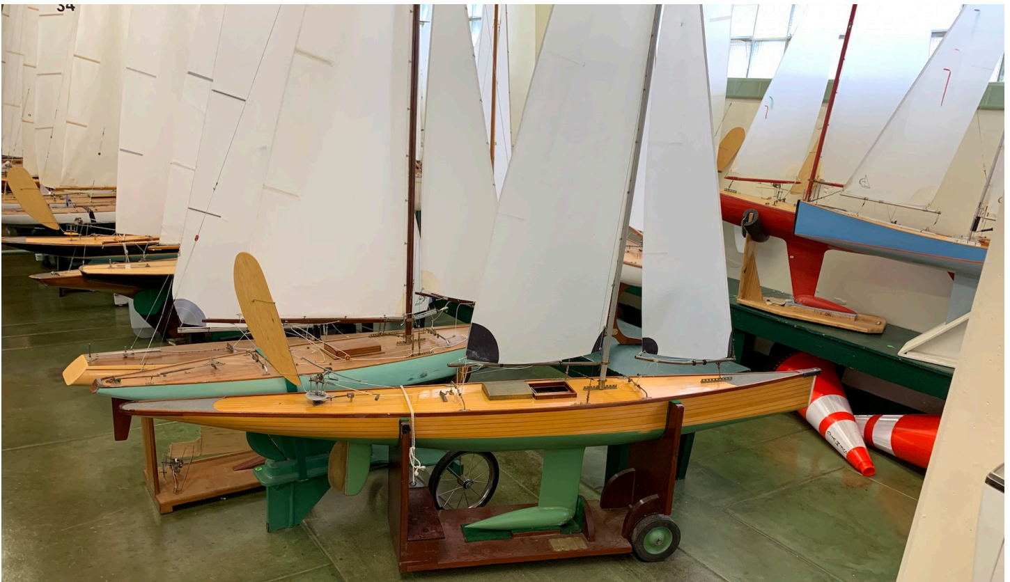
The elegant X Class was created in 1939 as an "experimental" class, to allow builders to try out different ideas. The rule sets a limit of 1,000 square inches of sail area (Ms are 800 inches), with almost no restrictions on hull shape, length, materials, or rig. It was a very popular class here at one time, as they have a lot of X woodies. I think the narrow one in the foreground got it pretty close to right, and I'd love to sail it with radio control and catch a blast reach – it would often be partially submerged and still track straight and fast. Bob Wells photo.
