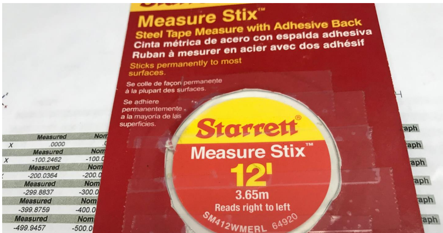
The measurement tape used on the tanks, with the accuracy certificate below. Ken Weeks photo.
