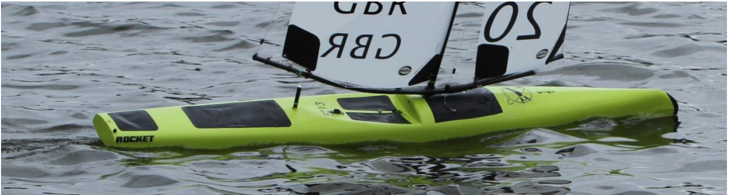
This caught my eye because of the wave piercing bow, very different from a few recent aggressively raised bows I see in IRSA Ms. With the rounded hull-deck edge to shed water this is super-clean and aero. Curiosity led me to modest Internet digging and the designer/builder is the UK's Mike Cooke. I wondered if he might have a rudder t-foil to resist diving, but an under-construction image on his website suggests none: https://www.facebook.com/aardvarktech/ . His Rocket Moths with the rigid wings are sensational to my eye, which knows little about Moths and Ms designs. With two lime-colored Rocket Ms sailing, maybe this will be another purchase option in this performance class? Sue Parkington image.
