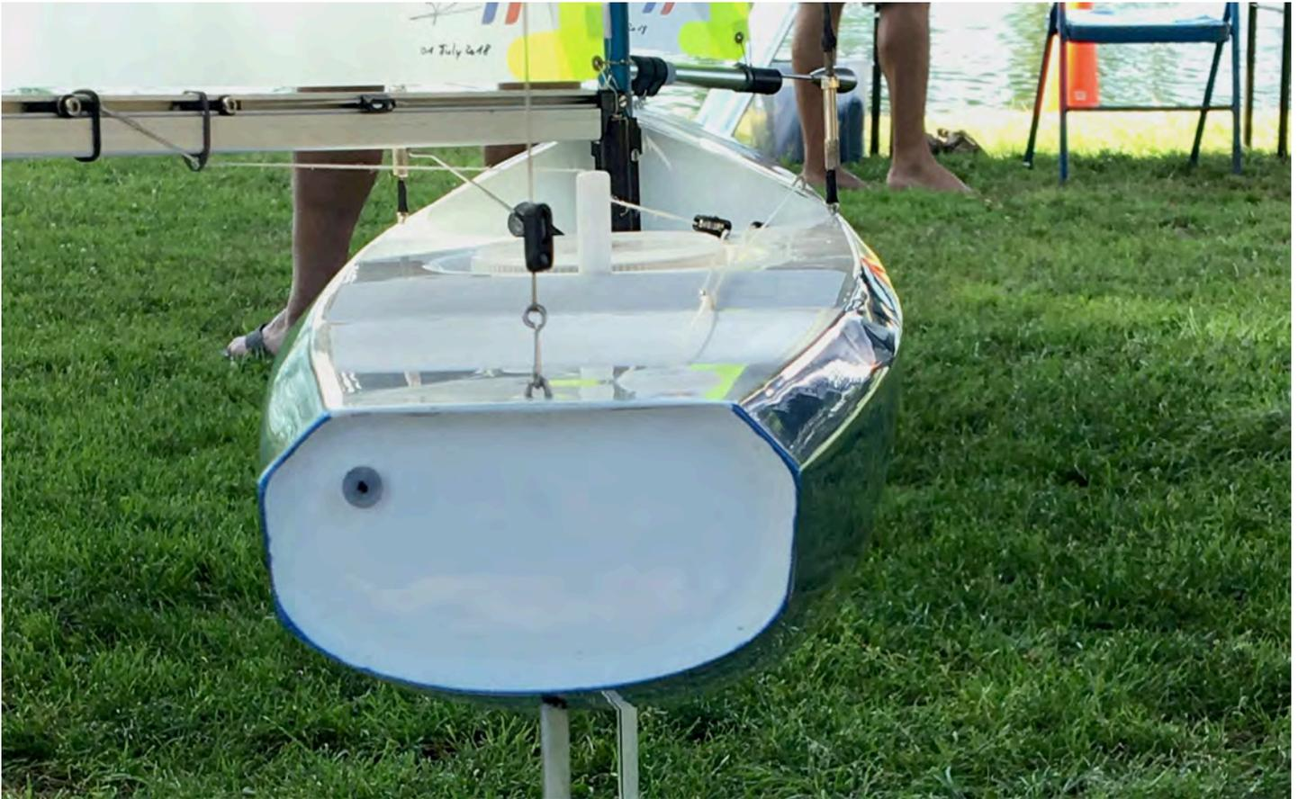
Stern view of Mikaël Pophillat's distinctive *Detox* with the chamfered hull-deck joint. We see rounded hull-deck joints all the time with hulls split down the middle in IOMs. Mikaël builds a separate deck where the join is an overlap at the chamfer. Bob Wells photo.
