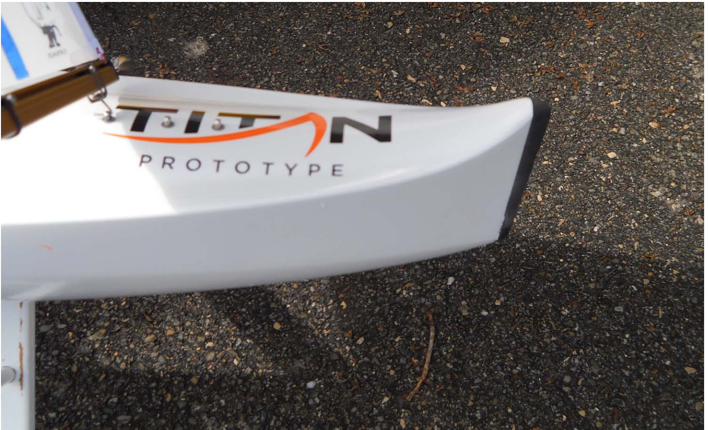
I know nothing of this proto sailed by France's Romain Dubreuil to 9 th place. That is one distinctive turned-up bow more commonly seen in the M class. Jerry Brower image.
