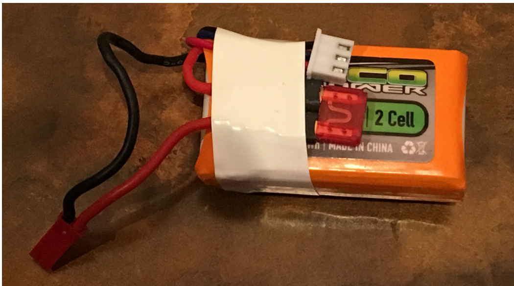
Joe's battery with tape in place ready to go in boat, and only the power plug is fully exposed. Bob Wells image.
