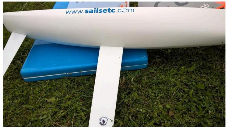
We were too busy sailin' so no images from our regatta. For grins let's see if you can name this intriguing yacht? Has SAILSetc branding... Has an emerging chine aft and flattish stern that looks overall wider than the Britpop! inspired hull forms... The hull has an emerging sharp "v" in the keel area instead of being rounded... Foils have short chords, which is very atypical of SAILSetc's usual Hollom designed foils. Need more clues – look below.
