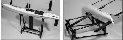
The Stand Upgrade Kit allows the boat to placed on the stand in the upright position for easy access when rigging and indoor storage (shown above left), or the stand can be laid on its side and the boat secured in an almost horizontal position (shown above right) for additional stability outdoors.
