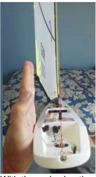
With the main sheeting angle set, the jib is then trimmed such that the hole in back of the jib boom fitting is over the first knuckle on the deck. It's close to 60mm between the middle of the mast and the inner edge of the boom.
