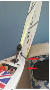
B rig: Backstay and mast: Bend that baby. Luff curve matches back of mast the entire length. Standard or 'stock' luff curve.
