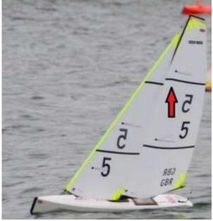
Mains twist. Finicky beast. Half a turn on the vang can make a surprising difference. I can only suggest a starting point and then fiddle with small changes until the boat looks and behaves to your preferences. Looking at the boat from behind when the boat is on the water and using the picture of John's boat as a template would be a good start.
