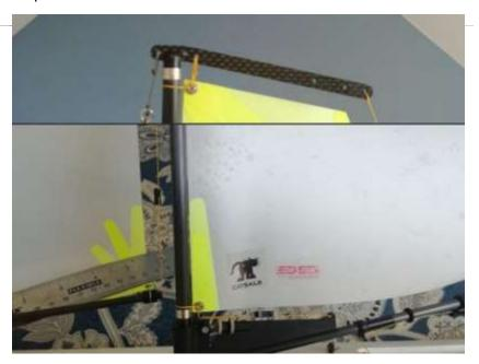
I run the mast gate as far back as possible and never touch it. It stays like this for all rigs. The DF seems to want as much aft rake as possible. So I rake it as far as it will go.
