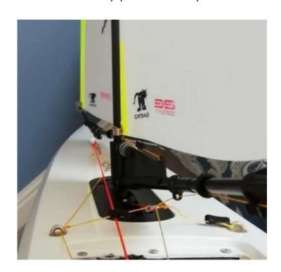
With a straight run for the jib sheet, it can get a bit snagged against the mast. Yes, jib fairlead is glued as well. I'll do a section on each rig, but the further forward you move the jib boom sheeting eye the further the jib will go out on the run. I've set my jib fairlead at 82mm from aft edge of joiner so that both the main and jib reach 90 degrees at the same time on the runs.
