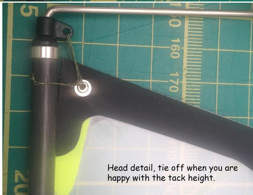
When you are happy with the height, tie off the head, then tie off the downhaul around the silicon ring.
