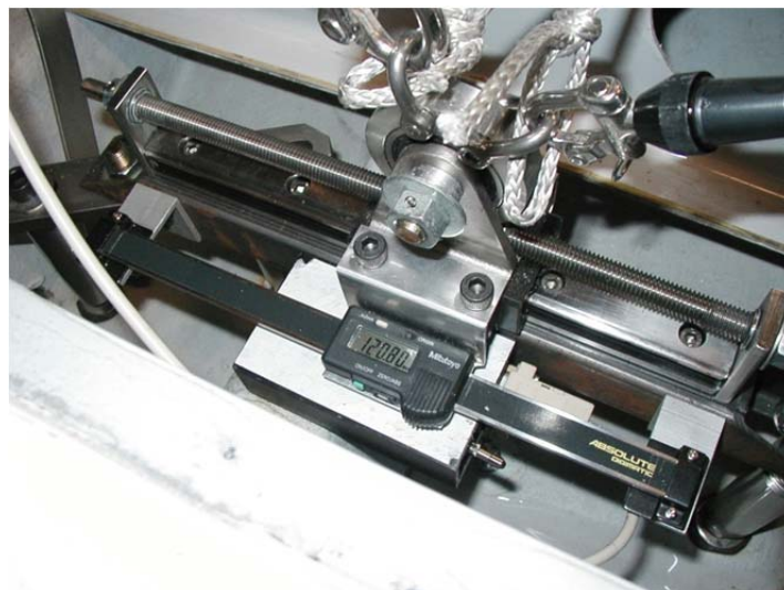
Figure H.4.7.2 The 2004 tilt swing system installed on the keel bolts of an Yngling. The swing bearing is mounted on a precision rail and the position read on the electronic scale. The box below the “rail scale” is the inclinometer. The roller bearing and the shackles for the support and steady lines of the suspension can be seen at the top of the photograph.
