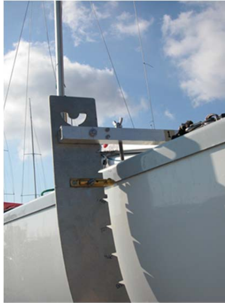
Figure H.1.5.1.1 The WS-produced Yngling templates showing the triangular cut outs at the measurement points and the lack of a reference line 10 mm from the template edge. The crossbeam and brass adjuster are essential added details. Note the locating pin, which precisely maintains the width of the template
