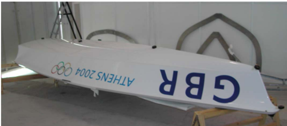
Figure H.7.1.1 49er with alignment pucks glued to surface.
