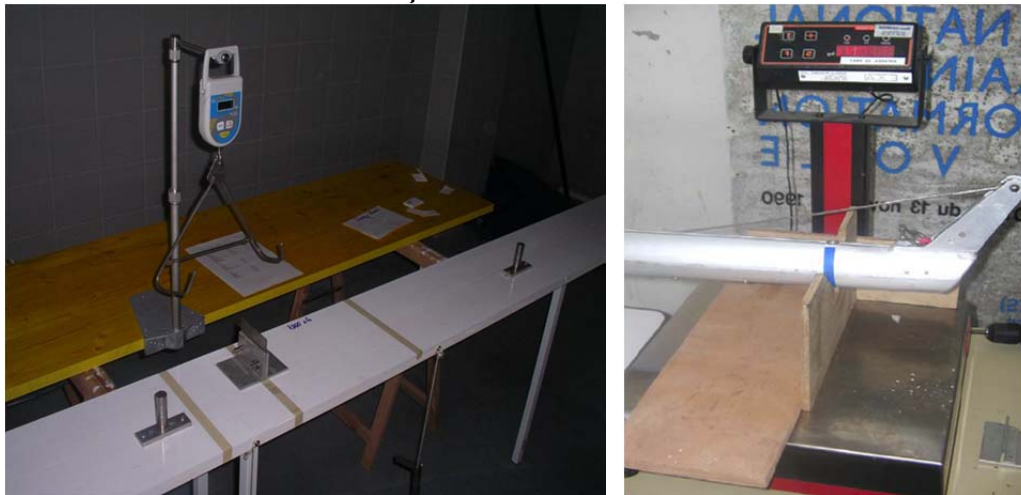
Mast weight / centre of gravity (left) and tip weight (right) measurement. The centre of gravity may be checked by using a knife-edge to balance the mast.
