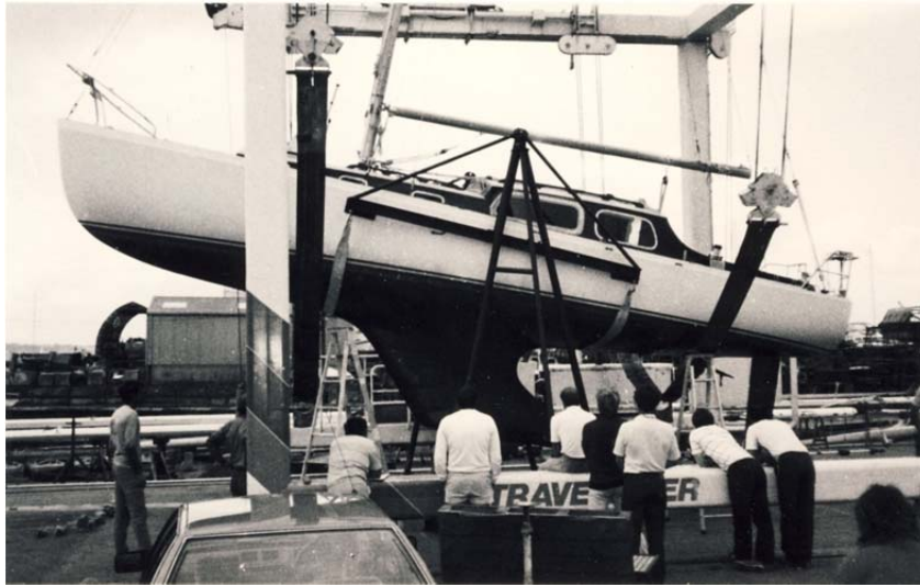
Figure H.4.6.1 A Stewart 34 undergoing a swing test in New Zealand in 1987.
