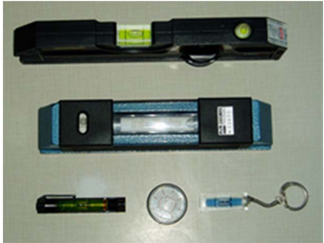
Figure F.6.5.1 A laser level, a 0.1 mm/m precision level, a hanging, a centre and a keychain level.
