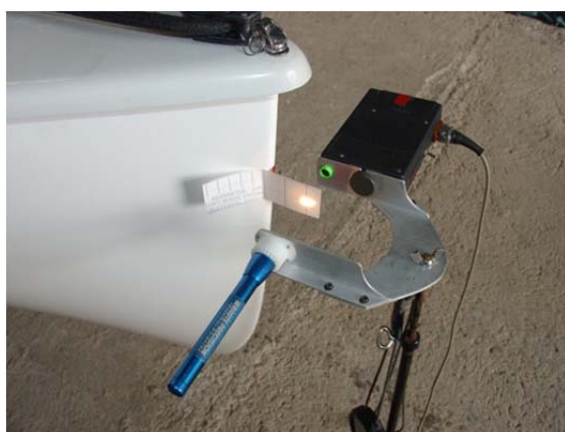
Figure H.4.2.1 A modern Finn Lamboley system showing the pairs of retractable knife edges, the Finn hooks with bearings 200 mm apart and the photocell used for timing.
