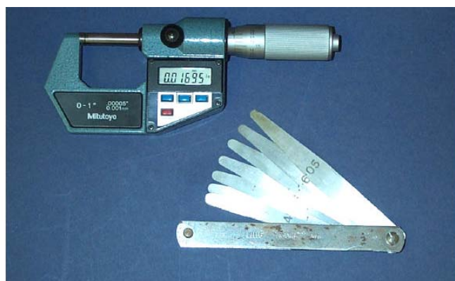
Figure K.1.2.3 A digital micrometre of resolution 0.001 mm and feeler gauges for sail cloth thickness measurement
